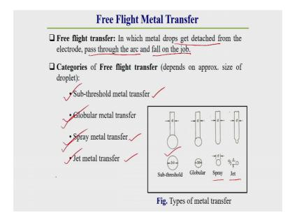
Generally free flight metal transfer what I have told you; that means, in which metal drops get detached from the electrode first, then is passed through the arc and fall on the job. So, what is happen here? Here generally drop get detached first, then pass through the arc and finally, fall on the gap. So, after detachment is freely fly in between gap that is why this welding this metal transfer is called free flight metal transfer.
