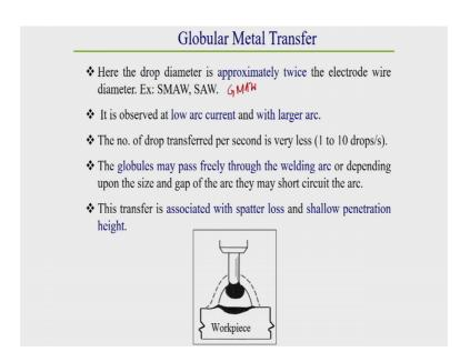
Generally globular metal transfer here the drop diameter is approximately twice the what I have already told you twice the electrode wire diameter. This generally we observed in case of submerged arc welding technique SMAW welding technique and GMAW also in GMAW welding process also; GMAW welding process also this types of drop transfer
