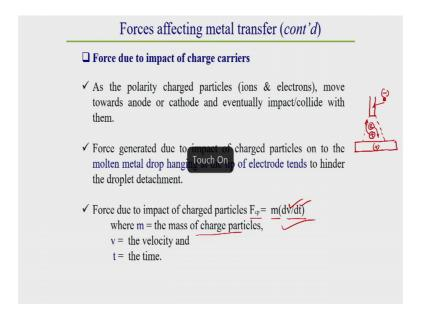
Now, we will see force due to impact of charge carriers. This force due to impact of charge carrier this is a happen, because what happens due to ionisation and emission of electron due to ionisation what happens in between this in between the gap of this in between the gap of this arc. So, in between this gap of this electrode and workpiece, what happens here generally develop electron and electron and ion?
