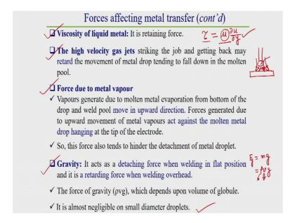
Now, we will go to other forces like viscosity of liquid metals. Generally viscosity due to the viscosity whatever the force generated in molten droplet that is generally also act as a retarding force. Because, generally we know from Newton's law of viscosity that we share new from Newton law of viscosity we know that shear stress between 2 adjacent layer is equal to viscosity into velocity gradient.
