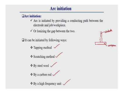
Generally arc is initiated by providing a conducting path between electrode and work piece. So, what happens for initiation of the arc let this is our work piece and this is electrode. So, first of all we have to make a conducting path actually by providing a conducting path that this is our work piece and this is our electrode.
