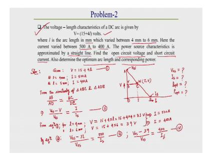
Here the problem statement is look like that is problem 2; the voltage length arc length characteristics of a DC is given by V is equal to this thing where 1 is arc length which is in millimetre which varied between 4 to 6 mm.
