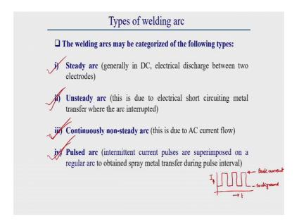
This four different categories of arc are this arc can be study arc that can be unsteady arc, this can be continuously non study arc and this can be pulsed arc. Generally a steady arc we observed in case of DC current where generally direct current power supply is used there we get a steady arc.
