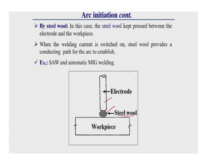
Then other technique like by steel wool in this technique what is done? Here a steel wool kept in between this electrode and work piece. Here you see this is the steel wool we generally kept in between this electrode and work piece; then current is switched on; that means, welding current is switched on.
