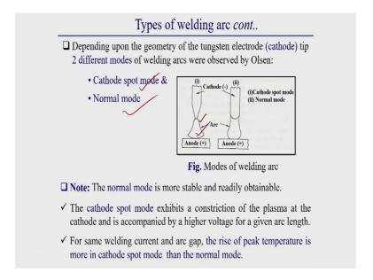
Here generally two different mode of arc we observe in case of tungsten electrode. So, here depending upon the geometry of the tungsten electrode here we observe two different types of mode of arc. What is these two different types of mode of arc? These two different types of mode or one mode of arc is called cathode sport mode arc, another mode of arc is called normal mode arc.
