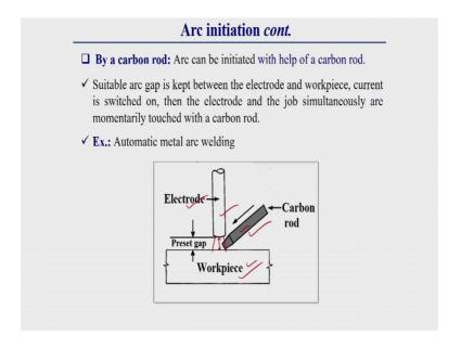
Then another categories is by generally a carbon rod also we can generate the arc; in this technique generally a suitable arc gap is maintained in between electrode and work piece this is the gap. Then the electrode and the job simultaneously momentarily toss with a carbon rod; so, first of all a gap is maintained then the current is 1.
