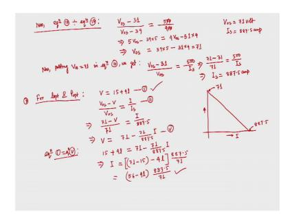
So, now by dividing the equation 3 by 4; so what we can write? Equation number 3 divided by equation number 4; by this what we can get? We can get V o s minus 31 divided by V o s minus 39 is equal to 500 divided by 400.
