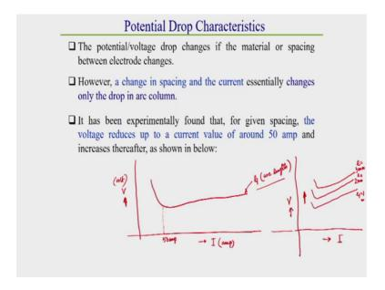
Here what we see for different arc length if the arc length increase then the voltage drop increase that we know; that means, arc length increase means gap increase gap increase means resistance increase because resistance is proportional to length. So, length increase voltage is also proportional to arc. So, what happens if the length increase arc gap increase then generally what happens voltage drop also increase in arc column.
