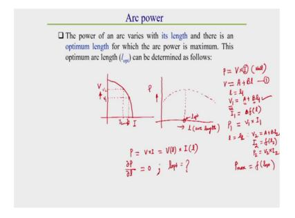
Now, we will go for how to find out the arc power; that means, so, arc power what is arc power arc power means we know that arc power is equal to voltage drop in arc column whatever that total voltage drop or welding that is that arc column whatever the total voltage drop is taken place or the that is called the welding voltage. So, arc power is equal to voltage drop in arc into supply of current from the power source; that means, this is called welding current.
