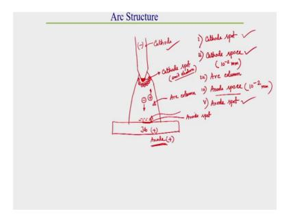
So, here what we observed last class, we have observed that this is a electrode this is a electrode and this is the work piece. So, generally electrode is cathode generally here let us electrode is cathode terminal cathode and work piece is this is job or work piece which is generally positive terminal; so this is generally called anode.
