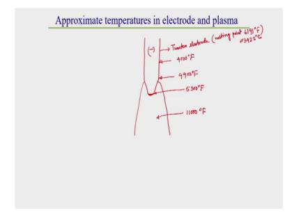
So, before going to this voltage drop change in arc column first of all here I will you should know actually what is the temperature distribution in a arc column as well as in electrode because that idea also here you should know. Because then also then only you will get some fairly good idea how much temperature generally generated in due to the due to a electric arc. Here just approximately I will just show you the how the temperature distribution in case of a GTAW welding process.
