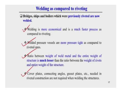
Earlier time bridges ships and boiler, which were previously reverted, are now welded; that means, earlier time generally bridge, ships, boiler, which were fabricated or manufactured by riveting, but nowadays that is replaced by welding process.
