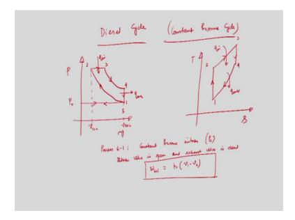
So, today I will discuss about Diesel cycle, and we will try to quantify the thermodynamic efficiency. Before, let me discuss you that since the constant combustion process is represented by a constant volume process, also the exhaust blow down that is a heat rejection is represented by constant volume process, Otto cycle is sometimes known as constant volume cycle.
