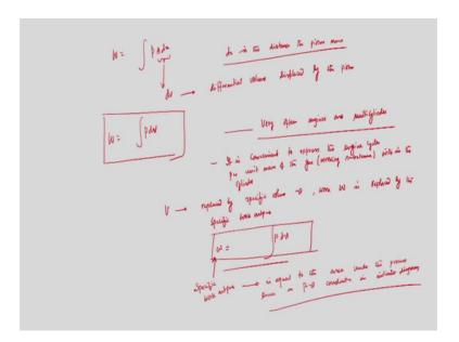
Now, so this is the work output from an engine that we are getting very importantly, this you know see A into dx, this is essentially dv this is volume that is the differential volume discussed by the piston. So, dv is the differential volume displaced by the piston right. So, W is equal to p dv p dv work that you are getting.
