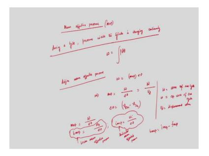
Mean effective pressure. So, this is known as mean effective pressure. So, what is the mean effective pressure? We have seen if I recall say if I go back to the you know actual p v diagram, we have seen that the pressure inside the cylinder is changing continuously it is not a fixed. So, pressure and volume rather it is a you know continuously changing right. So, this is the cycle, during a cycle pressure inside the cylinder is changing continuously, this is very important.
