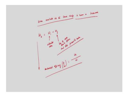
That means work available at the crank shaft at the crank shaft work available at the crank shaft is known as brake work brake work w b. So, w brake is equal to w indicated, I am writing the you know I am writing the specific work available at the crank shaft at the crank shaft is known as brake work, and that will be w indicated minus w f.
