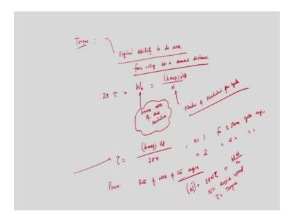
Now, I will discuss I what is torque and power because again we need to calculate torque. Torque is a good indicator of an engine ability to do work right. What is torque;
