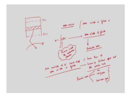
Next I would like to discuss that again if I draw the again you know engine cylinder, this is very important. So, if I draw the engine cylinder, suppose this is this piston, and this is TDC, this is BDC, and piston will move in this direction. So, we may have you know air supply I am not going to draw the supply line of air exhaust manifold all those things, but this is the indicator this is the engine cylinder.
