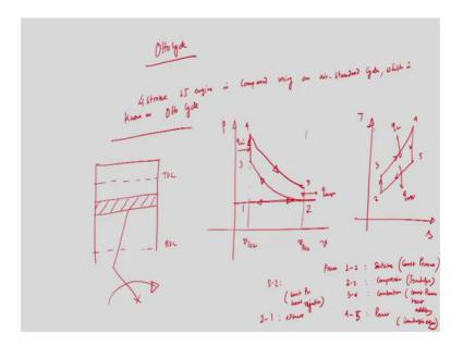
So, I will take about Otto cycle. So, what is Otto cycle? As I said you that whenever we are talking about four stroke engine and two stroke engine we have discussed in detail about four different strokes and two different strokes. So, normally we cannot call it as a thermodynamic cycle that is what also we have discussed is a mechanical cycle, but essentially we have seen that the pressure and temperature is continuously changing in a cycle.
