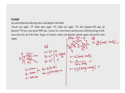
So, after this we will see an example for the typical turbine case and then example reads like, an axial turbine as following data at the mid height of the blade. We should remember this example is purposely chosen for the fact that we had seen something which is called as the radial equilibrium and free vortex theory. So, this example is based on that free vortex theory and radial equilibrium. It helps us to understand different concepts.
