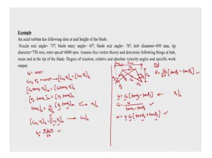
So, we will take C a is equal to constant. This is known to us we take it to have no axial thrust and then we are knowing that C w 2 into r 2 is equal to constant by all these means we mean C w 2 into r 2 for the mid is equal to C w 2 into r 2 at hub.
