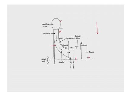
Now, same way as we had axial flow compressor and radial flow compressor which is a centrifugal compressor we have axial flow turbines and radial flow turbines. So, in the radial flow turbines unlike axial compressor where we had a flow which is going outward and we are having which is flow coming inward. So, inward radial flow turbines. So, are generally worked out in the incompressible flow regimes. So, the gases generally have inward radial flow turbines.
