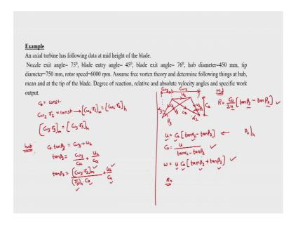
So, at hub we know that. So, this is one thing. So, we can we need to find out beta 3. So, we can say that u C a into tan beta 3 at hub we are doing it for hub, but velocity triangle can be similar. So, we will say C a into tan beta 3 at hub is equal to C w 3 plus C u 2. So, basically this is what C a tan beta 3. So, we have tan beta 3 is equal to C w 3 upon C a plus u 2 upon C a.
