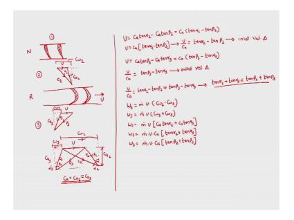
So, now having said this, we will see now how we can draw the velocity triangles for the general gas turbine, which would be either impulse or reaction. So, let us draw a schematic of the first nozzle. So, let us say we are working with the nozzle, so let us draw a schematic of the nozzle.
