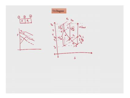
So, now next point to be discussed is the T-S diagram or the axial turbine. So, for T-S diagram, we know that we will write down our schematic as what we did for the compressor, we first have nozzle, then we have rotor, 1 to 2 is nozzle and then 2 to 3 is this rotor. So, we know that what is going to happen in turbine.
