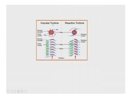
So, as what we would see that there are two components two types of turbines, which are gas turbines; one type of gas turbine is called an impulse turbine and other type of gas turbine is called as a reaction type of gas turbine. So, in these gas turbines as what we had seen, there is nozzle which is green in colour, then there is rotor which is red in colour. In the same case, here as well in reaction turbine green is the stator or the nozzle, and red is the rotor.
