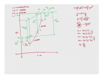
So, let us continue that and then see. So, we have flow which is i to 1 then 1 to 2 and then 2 to 3. Here the flow is between accelerate in nozzle flow is between nozzle and inlet guide vanes it is in the impeller and it is in the diffuser. So, i to 1 1 to 2 and 2 to 3; so this is our flow passage. So, for that all let us try to draw the TS diagram.
