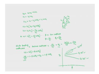
We had written down w s stage is equal to u 2 cw 2 minus u 1 cw 1 when we say that we will neglect the inlets well we will we say that ws is equal to u 2 cw 2. And if we go back and find out what is cw 2; if we try to find out what is cw 2 then we will go back and see what is cw 2. So, what is c w 2? c w 2 is this; so if you take a typical case of backward facing vane then c w 2 is u 2 minus this. So, c w 2 we will write down this velocity triangle here.
