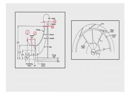
So, if we go back and then see if we go back and see the; see the diagram what we had seen earlier which is the configuration of the centrifugal compressor; where we can see that this is the I inlet of the centrifugal compressor. And then till this point from here to here we have the inlet accelerating nozzle from here to here we have inlet guide vane.
