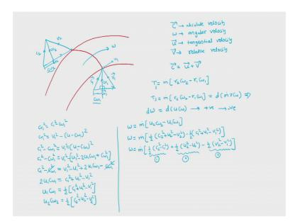
And as per that velocity triangle let us consider that, a general turbo machine, in that turbo machine this is the blade having this blade with us we will have this something as inlet. So, for that inlet we will have this as the velocity which is the relative velocity, this will be absolute velocity and then this will be the tangential velocity and this will be the radial velocity C r 1 ok.
