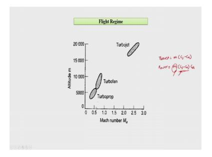
Then we have Flight Regimes. What we have talked till time was about the application and different arrangements of the turbojet or turbo based engines or aircraft engine, but the turbo engines which is turboprop, turbofan and turbojet as what we have seen if we remember there we have said that there is thrust which is m dot c j minus c a and then there is power which is based upon thrust which is m dot c j minus c a into c a.
