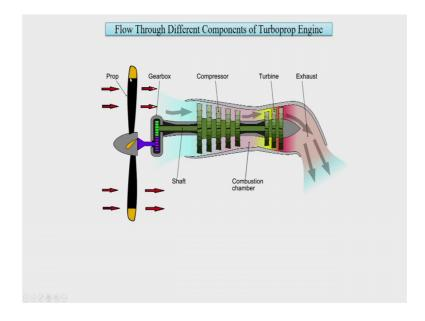
So, practically what would happen in case of turbofan engine is there would be turboprop engine, is there would be a propeller which is basically the driving mechanism, propulsion mechanism for the getting thrust. So, these needs to be rotated. So, since this is needing to be rotated first air would pass over it.
