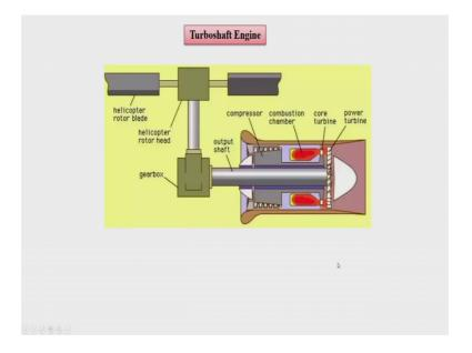
Then what we have is a Turboshaft arrangement. Turboshaft arrangement is what we can have it in the helicopter. Turboshaft arrangement is not different from the arrangement what we generally have in case of the electricity based gas turbine power plant where shaft is connected to a gearbox, shaft is connected to a generator, but in this case the gas turbine power plant is connected to a shaft and that shaft is going to rotate the blades of the helicopter.
