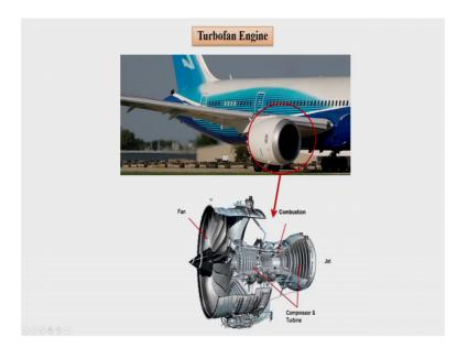
Say then now next engine is Turbofan Engine. Turbojet engine as it was suggested that whole thrust was obtained from the jet. So, j c j is very high and across that c j we are having extra thrust. So, now, we have an engine which is called as turbofan engine where not all thrust is obtained from the jet there is some thrust which is obtained from the other part of the engine where air is not combusted.
