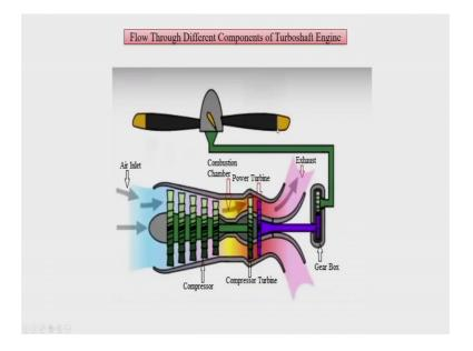
Here the arrangement of turboshaft engine is same way as what we have in a general or conventional turbojet engine except that the shaft which is connected to the turbine is also connected to the gearbox. So, turbine runs the gearbox and hence the propeller. So, practically turbine drives the compressor and propeller both in case of a Turboshaft engine.
