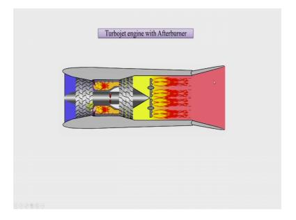
Then in case of turbojet engine there is one more entity, which is called as after burner once the flow passes from the compressor combustion chamber and turbine it is expected to expand, but there is some amount of oxygen which is unburnt here since most of the time this combustion whatever it would take place it would take place in the lean range. So, fuel is a lean less and then a oxidizer is more.
