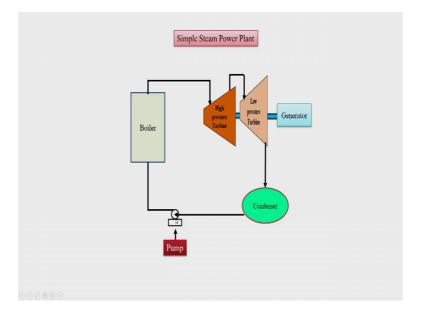
So, first we will see what do we mean by a steam power plant. In a steam power plant as we know we have high pressure and high temperature steam stored in the boiler, and this steam would go over the high pressure turbine. And then high pressure turbine exhaust is
