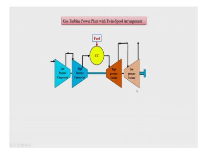
So, how would be the arrangement, in case of two spool arrangement, we have low pressure compressor, and we have low pressure turbine connected with a shaft. But then, we have high pressure compressor, we have high pressure turbine connected with some other shaft. So, these shaft will pass inside each other. So, this is an hollow shaft which is connecting high pressure compressor and high pressure turbine, which is again having a low pressure connection passing through it.
