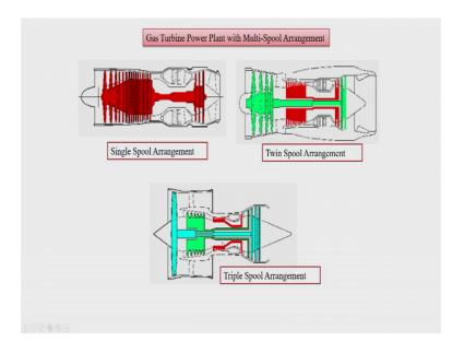
So, we have multi-spool arrangement as what we can see single spool arrangement. This is a single spool arrangement where there is a compressor. It is connected with a turbine using the single shaft. So, there is only one shaft. So, this is turbine, this is compressor, they are connected by single shaft. So, it is called as single spool arrangement.
