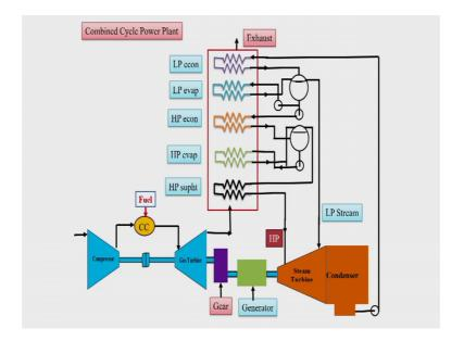
But then, when we see that we want to increase the efficiency of our gas turbine power plant. We can think of it to be coupled with a steam power plant. So, this is a little complicated diagram, but let us see how the passage is for the gas and how it helps us.
