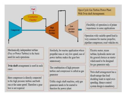
In case of twin shaft arrangement again we have compressor we have combustion chamber, we have turbine and turbine high pressure turbine and compressor they are connected by one shaft, but exhaust of this turbine is given to the low pressure turbine which is run by a separate shaft. So, there is a separate shaft for the low pressure turbine, but high pressure turbine drives the compressor. So, this is what called as the twin shaft arrangement of a gas turbine power plant.
