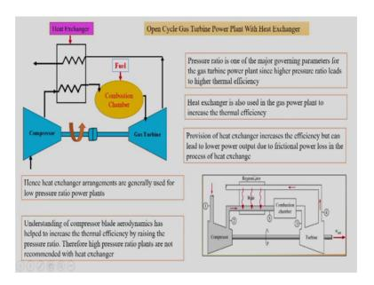
So, we have now come to a point that we want to increase the efficiency. One way what we have said that we can increase the efficiency by increasing the pressure ratio of the
