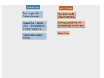
And, we have in reaction turbines there is a certain difference between impulse and reaction turbines. So, in case of impulse turbines we have seen that there is energy transfer in the rotor and they are having constant area passage. But, in case of reaction turbine there is energy transfer and energy transformation in the rotor since the rotor blades are having a passage which is a converging duct.
