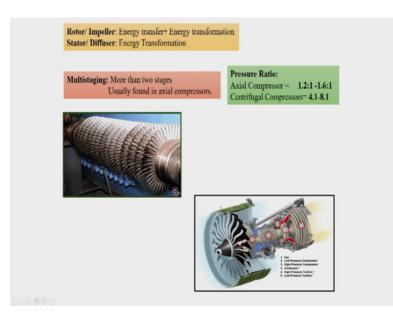
So, as we have seen there is a rotor in centrifugal compressor or in case of axial compressor it would have done two jobs. First job is to transfer energy, as we know that their rotors energy will get transfer to the fluid. But, apart from that internal arrangement of the rotor blades would also lead to energy transformation. Here we mean bi energy transformation that one form of the energy will get converted into other form of energy.
