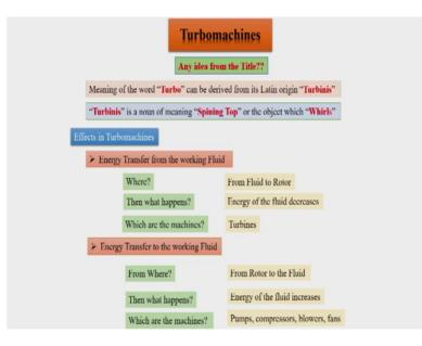
The title turbomachine has it is connection with the latin word terbinis. Terbinis is a latin word which is a noun and its meaning is spinning top or the object which whirls; that means, which rotates. So, turbomachines would deal with the machines which are rotating machines or the machines in which the parts of it are rotating; so this is what the turbo machine definition is.
