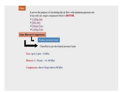
Turbomachine as what we have seen a kind of fan we have seen that the fans are the turbomachine. So, here we are starting first for fan, it is a simple turbomachine and it has only one component and that is rotor. Fans basically lead to a minimal or a small amount of pressure rise.
