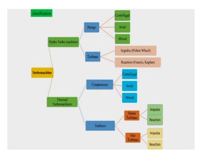
Then we have classification of all the turbomachines. So, turbomachines can be broadly classified into two categories; one is hydro turbomachinery and other is thermal turbomacineries. So, in hydro turbomachineries as we know we have pumps and turbines. In thermal turbomachineries we have compressors. Basically pumps do a job which is getting then in thermo machineries by compressors and the second is again turbines.
