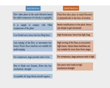
So, what is the difference or advantage between axial flow machines and the radial flow machines. So, as we have seen this difference is for let it be compressor or let it be turbine.
