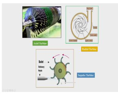
So, this is axial flow turbine pictorial view and this is radial flow turbine and then as we know in case of water this is an impulse turbine. This is a principal demonstration for an impulse turbine.
