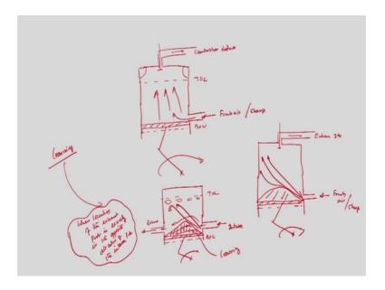
So, if it is schematic of SI 2-stroke engine, suppose as I said you sometimes you know. So, I am trying to define cases. So, this is either fresh air or charge. Now so, this is lets this is piston and this is BDC and this is TDC and this is combustion product.
