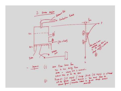
So, if I draw a schematic of a two-stroke engine; so, 2-stroke engine. So, if I draw the 2-stroke engine we have this is top dead center and this is bottom dead center right, and we have piston. So, I am giving if it is so, this is intake port, this is exhaust port through which combustion product go out.
