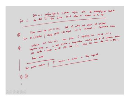
And this is known as this is uniflow type, this is very important I am underlying this line uniflow type of, this is a uniflow type of 2-stroke engine since, since the scavenging air tends to flow in 1 direction that is from intake at the bottom full exist in the top. Since this scavenging air tends to flow, tends to flow in one direction in one direction that is from intake at the bottom to top to the exhaust at the top exhaust at the top.
