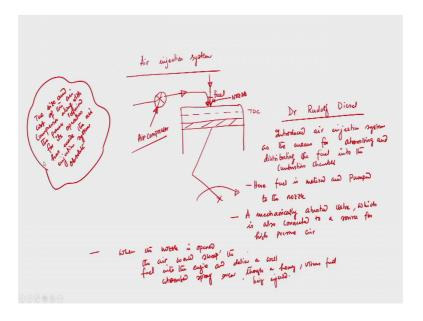
Schematically I will show. So, we suppose this is a engine cylinder, this is stopped at center, we need to supply fuel over here, and then we have one air compressor, and then this compressed air is taken over here. So, this is air compressor.
