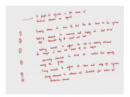
So therefore, I can write now. Therefore, to fulfill the objectives of few number of functional elements are required, right. So, number 1: what is number of objective meter the quantity of fuel, right. Meter the quantity of fuel demanded by the load and speed of
