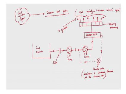
So that means, in a air a solid injection system we have it can be sub classified into three categories: common rail system, individual pump, and nozzle then unit injectors.
