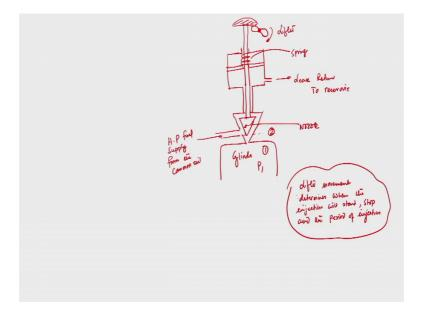
So, this is one. So, this is a schematic nozzle, so it take high pressure supply from that common rail, then it you know it strikes the nozzle you know nozzle face. Then this nozzle is connected with a spring you know loaded spring, so this lift is there one this is
