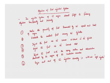
Objective of fuel injection system right. So, the injection system of CI engines should fulfill the following: I mean I can write the injection system of CI engine should fulfill the following objectives consistently and precisely; consistently and precisely, right. Number 1 is: meter the quantity meter the quantity of fuel demanded by the speed and load of the engine this is very important. Meter the quantity of fuel demanded by the speed and load of engine. Number 2: distribute.
