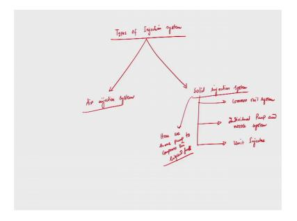
So, types of injection system. This is classified into two category: first one is, air injection system. And number 2 is, solid injection system. This is further classified into three different categories: first one is you know common rail system, individual pump and nozzle system, and last one is unit injectors.
