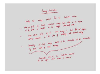
So, I can write that heat energy distribution. So, mostly the energy produced from the combustion reaction. Now 35 percent of the total chemical energy of total chemical energy that; enters an engine in the fuel that enters an engine in the fuel. In the engine in an in an engine in the fuel in an engine is converted to the useful crankshaft work.
