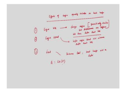
So, I mean size speed so I mean what are the effects of engine operating. So, effects of engine operating variables on heat transfer on heat transfer. So, basically engine size first one is engine size is very important engine size. So, it everything is remaining same to geometrically similar engine of different size different displacement.
