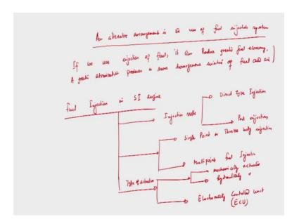
And to an alternative arrangement an alternative arrangement, is the use of fuel injection system. So, alternative arrangement is the use of fuel injection system. And that means, if we use you know injection of fuel injection of fuel it can produce greater fuel economy. Greater atomization greater atomization produces more homogeneous mixture of fuel and air. It is very important.
