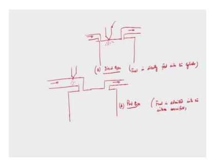
So, this is direct type. So, this is exhaust manifold this is intake manifold this is fuel injector of fuel nozzle through which fuel is injected. So, direct type fuel is directly fed into the cylinder fuel is directly fed into the cylinder right. Or if it is port injection fuel is admitted into the intake manifold.
