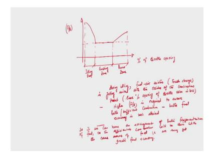
And this is one problem. Another problem is if you try to recall our you know fuel air ratio versus first you know if you try to recall that, 3 different zones of engine operation that is if I have fuel air ratio and this is percentage of throttle opening, then most of the time although engine is running you know in crushing zone, but still we have. So, this is idling zone, this is crushing zone, this is powered zone.
