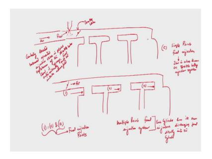
Now, we will see the single point fuel injection system as I said that, if we have a multi if we have a multi cylinder engine. So, we can supply fuel over here; so this is fuel, and air is going over here, this is fuel this is air. So, this is c single point fuel injection. This is single point fuel injection.
