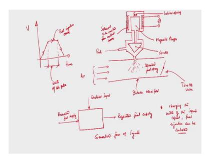
Now, multiple fuel injection; so here we have seen that each cylinder has it own injector discharging fuel into the cylinder. Now we will discuss about very important that what is you know mechanical. So, if I now draw; suppose we have we are supplying fuel into the intake manifold. So, this is intake manifold air is coming. So, this is air, this is intake manifold right. And we have a throttle valve so this is throttle valve.
