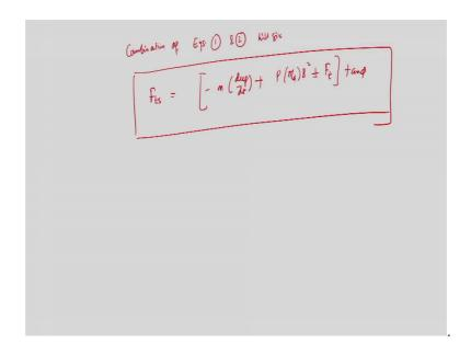
So, now, if I combine equation 1 and 2 so, combination of equation 1 and 2 will give that F ts that equal to minus m du p dt plus P in to pi by 4 B square plus minus F t into tan phi. So, this is the expression of the side thrust force that depends upon the pressure inside the cylinder, frictional forces and also the acceleration and phi angle. So, I mean so, this is the side thrust phase which is acting this only because of the rotation of the piston between 2 locations TDC and VDC.
