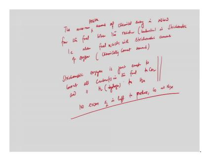
So, the maximum possible amount of chemical energy so, the maximum as I said that, we would like to maximize the energy conversion rate during the combustion reaction. So, the maximum amount of maximum possible amount of energy conversion or chemical energy is obtained from the fuel. So, as I said that since there are thousands of hydrocarbons so and which consists hydrogen, carbon mainly and up to some extent oxygen, sulphur, nitrogen.
