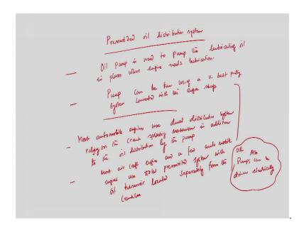
Pressurized oil distribution system, so, for this pressurized oil distribution system rather pressurized lubrication lubricating lubrication system a pump is essential. So, oil pump is used to pump the lubricating oil in places where engine needs engine lubrication we have to supply this is very important. And sometimes this pump is we have discussed that for the cooling system sometimes we there are 2 different types of cooling system, air cooling air cooled engine or water cooled engine.
