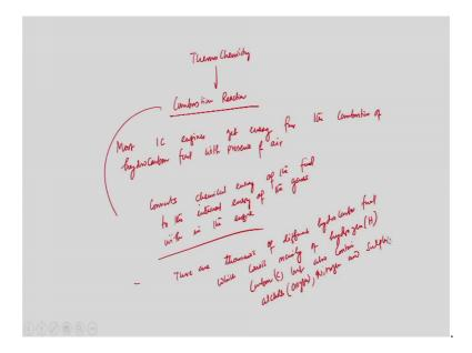
So, essentially this gives us an information about the combustion reaction very important that because most of the IC, most of the engines or internal combustion engines most internal combustion engines you know get energy from the combustion; from the combustion of hydrocarbon fuel with air with presence of air.
