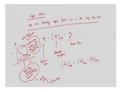
So, what we can do that in engine friction. Very important that engine friction is very important that friction can be classified you know rather we can classify engine friction we can classify engine friction as a loss using power terms. So, essentially friction is loss of power right because a significant portion of the power is required to overcome that frictional losses.
