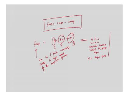
So, that is why I can write that frictional mean effective pressure is equal to indicated mean effective pressure minus break mean effective pressure. So, that is what I can write that is very important. that frictional mean effective pressure is equal to indicated mean
