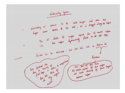
So, when one surface move relative. Suppose we have a lubricating system. So, we have understood that why we need lubricating system in an internal combustion engine. So, lubricating system is nothing, but a system where we can have lubrication oil either we can pump the lubricating oil to the desired locations of the internal combustion engine. Or sometimes the movement of the crank shaft itself allows the you know charging action of the lubrication lubricating oil.
