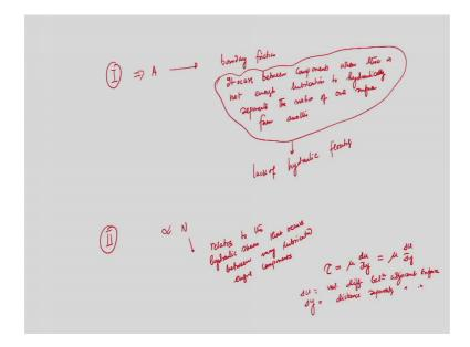
So, this first term a first term that is a it is very important is known as boundary friction this is known as boundary friction very important. So, it occurs between components. So, boundary friction and it occurs between components when there is not enough lubrication to hydraulically separate. So, there is not enough lubrication to hydraulically separate the motion of one surface from another.
