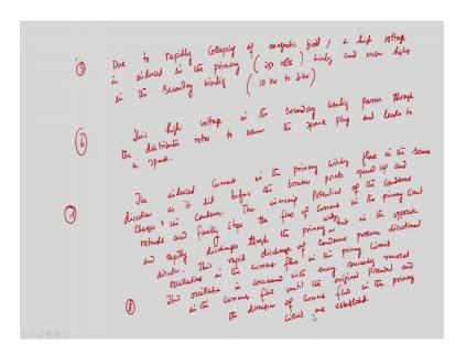
Now very importantly, number 4 number 5, number 5 due to rapidly collapsing due to rapidly collapsing of the magnetic field rapidly collapsing of the magnetic field, a high voltage is induced in the primary; a high voltage is induced in the primary, which is of the order of 25 2 5 about 250 volts. Primary winding and even higher in the even higher in the secondary windings; secondary winding even in the higher and the secondary winding, which is of the order of 10 kilovolt to 20 kilovolt.
