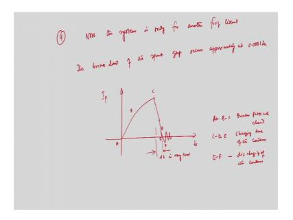
So now, 9 now the system is ready for the system is ready for the for another firing circuit, for another firing circuit very important. The enter break down process usually takes very small second of the order of 10 power minus 3 10 power minus 4 second. The breakdown of the spark gap; the breakdown of the spark gap usually occur approximately at 0.0001 second.
