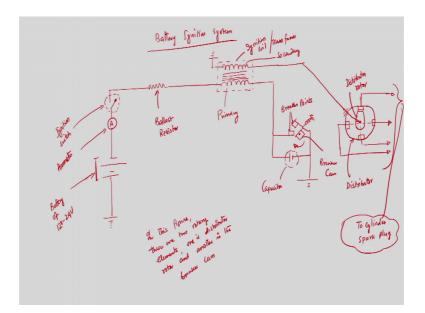
So, this is a schematic we have discussed about the function of each and every you know parts of the system. We have ignition switch and then we have register and ignition coil and breaker points and distributor rotor.
