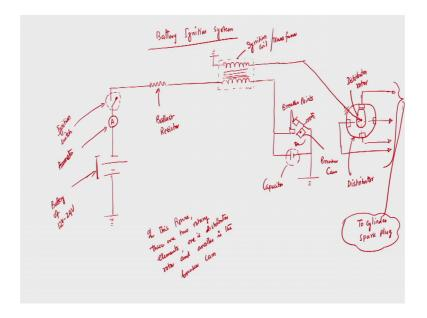
So, if I try to draw the schematic of a spark ignition rather battery ignition system. So, schematic of a battery ignition system. So, this is battery ignition system. So, if I try to draw the schematic. So, will have a battery. So, then we have an ammeter connected, then we will have a ignition switch, then we have one register, then we have one transformer, which is having primary and secondary circuit.
