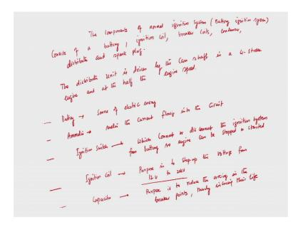
So, now question is the component what you have drawn. So, the components you know of the normal ignition system consists of a battery, the components of normal ignition system that is battery ignition system consists of a battery that is source of electrical energy battery, ignition coil, ignition coil, breaker coils, condenser, distributor and spark plug, condenser, distributor and spark plug.
