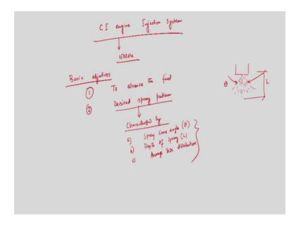
So, in general nozzles are used in a CI engine injection system. So, if I tried to talk about nozzle, then preferably nozzles are used in a CI engine, compression ignition engine, injection system. So, basic objective CI engine injection system. Whenever, we are thinking about the injection system rather we are going to discuss about the injection system in a compression injection engine, of course we cannot nozzle is an integral part of that.
