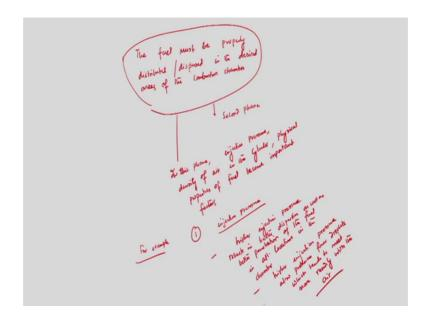
Second objective we will discuss that the fuel must be, the fuel must be you know properly distributed or dispersed in the desired areas of the chamber. Fuel must be properly distributed or dispersed in the desired areas of the chamber; in the desired area of the combustion chamber.
