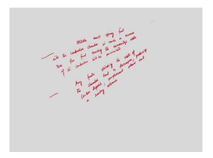
So, now we will come to the discussion. So, from this discussion, we have seen that the nozzle must spray fuel the chamber in such a manner. So, from the discussion we have seen that that nozzle must spray the fuel nozzle must spray fuel into the combustion chamber in such a manner, in such a manner that the you know that the fuel reaching the surrounding walls surrounding walls of the combustion chamber.
