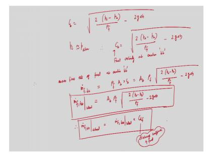
Therefore we have obtained the velocity of fuel at section b b that is C b is equal to twice into p c minus p b divided by rho f minus twice into g into delta h under root. Note that p c is almost equal to p c is equal to atmospheric pressure p atm. Therefore, I can write C b is equal to twice p atmospheric minus twice p b divided by rho f minus twice g into delta h that is the velocity of. So, this is the fuel velocity at section b b.
