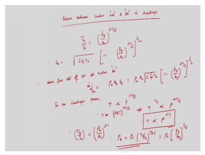
So, we can assume the process between section a a and b b is isentropic. So, process between section a a and b b is isentropic this is not again a very bad assumptions because there is no heat interaction between the between these two section and also the frictional
