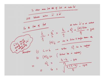
Now, to obtain mass flow rate of fuel at section b b, we have to apply steady flow energy equation between section bb and section cc. So, we are applying steady flow energy equation between section cc and bb.
