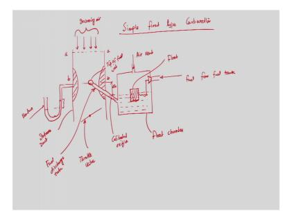
So, today I will discuss about a simple float type carburettor. Although these are not used nowadays, but still only to have a under only to have an understanding about only to have understanding about the you know processes which is there in a carburettor, how a carburettor is supplying air fuel ratio or fuel air mixture depending upon the requirement of the engine load; we should discuss this in detail.
