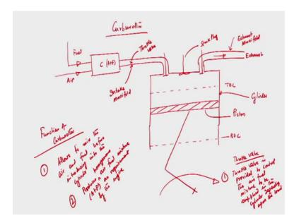
Today, we will discuss about Carburettor and which is an important part of SI engine. So, we are having instead of supplying only air, suppose this is carburettor c. So, we are having ah, we are having supply of fuel and supply of air.
