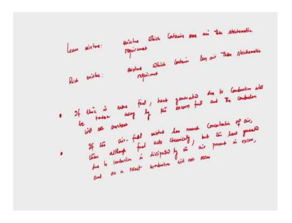
So, there I have discussed, I have written the lean mixture and rich mixture what is lean mixture? Mixture which contains more air than stoichiometric ratio. So, lean mixture; lean mixture the mixture which contains more air than stoichiometric, than stoichiometric ratio stoichiometric requirement.
