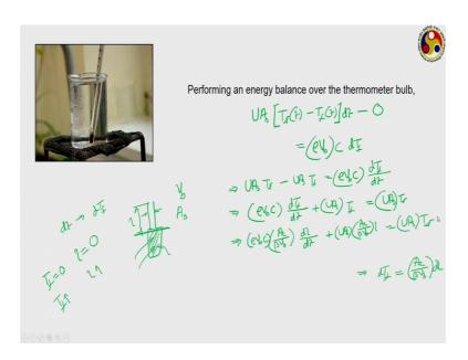
So, let us replace this one in the earlier equation. So, if we go back to the earlier equation, then we have row V b C into from here we can also write that d T f will be equal to A c upon beta V b into d l. So, putting it there we have A c upon beta V b into d l d t plus original equation at U A s into AC upon beta V b into l of course is equal to U A s T infinity.
