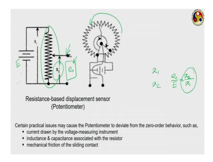
Something that very closely resembles the input is the resistance based displacement sensor called the potentiometer. In the concerned model, we shall be discussing a bit more about potentiometer. But, the principle of potentiometer is that here you have a resistance like this which is being subjected to which is being excited by a constant voltage source kept here.
