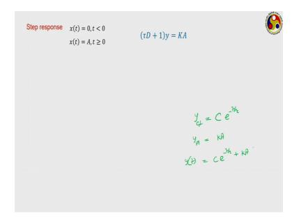
So, first you check the step response, we know this is the step response. So, how to do it? We know for a first-order system, this is the way this is the standard form here K is the static sensitivity, and A is the input that you are giving for any value of tau or sorry any value of time greater than 0. So, we have to solve it.
