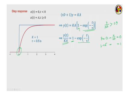
You can clearly see, there are two parts of this solution. One is this 1 which is a constant value, and other is this particular quantity. We can explain it bit more, if you represent the solution in this form. Here we are dividing the output by K into A thereby making it non-dimensional. Look at this here one this term is 1 which represent the constant, and what about this term this is an exponential term which an exponential term negative exponential term.
