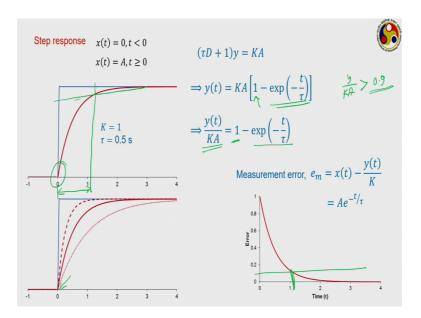
The measurement error is often referred as the input minus this y upon K quantity. So, in this case it will be A into e t upon tau. And if we plot that with time, you can see that initially your measurement error is 1 which is referring to this particular point. And as the time goes on the error keeps on reducing.
