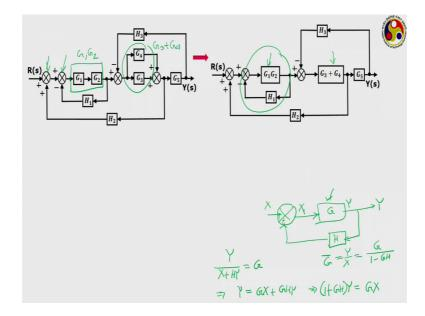
So, using this particular knowledge, we can clearly say that like say for this particular assembly our equivalent transfer function will be G 1 into G 2, whereas for this particular assembly our equivalent transfer function will be G 3 plus G 4, and that is what we have here G 1 into G 2 here replacing the G 1 and G 2 individual components and here again G 3 plus G 4 replacing the individual components.
