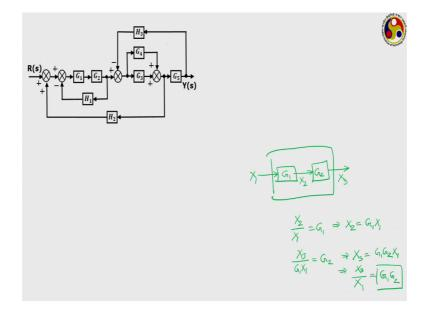
First possibility let me erase it make it a bit cleaner first possibility is where we have two components connect in series. Connect in series means, the output from the first component is directly fed to the second component. Like if the first one is having output G 1, second one is having sorry first one is having transfer function G 1, second one is having transfer function G 2.
