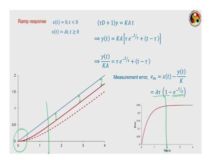
So, this is the corresponding error, you can see the error initially is 0 here. And then it keeps on increasing, and then becomes constant beyond a certain time for this. So, this is a step and ramp response, we shall be talking a bit more on them in the next lecture, and we shall also be checking out the response of a first-order system in terms of impulse and frequency response.
