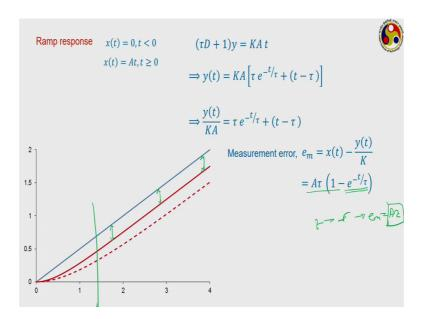
We shall be checking other response today that is the ramp response we know this is the form of the ramp. So, we this is the corresponding function of functional form. And if you solve this on following again the complementary function and particular integral, we are going to get a solution of this particular form where we again have two parts. Both cases the tau is involved.
