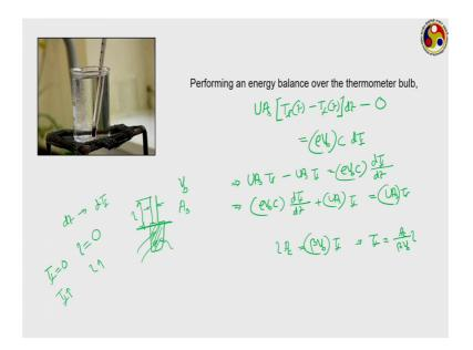
Now, example for first-order system, there are several most common one is a liquid in glass thermometer. There can be other examples like one capacitor discharging current through a resistor, there can be one tank of water leaking through a wall, these are all very common examples of first-order system. We shall be seeing a few more examples later on, let us just concentrate on this one.
