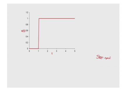
Let me take another signal. This is a particular type of signal, which we have to use quite a bit more. These are known as step signal or step input. Step refers to just a single step change in the input, here like the situation shown here till a certain time the input signal was 0.
