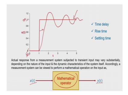
Actual response that we are going to get from a measurement system, when that is subjected to a transient response or transient input I should say that can vary substantially depending on the nature of the input that you are providing, and also the dynamic characteristic of the system itself.
