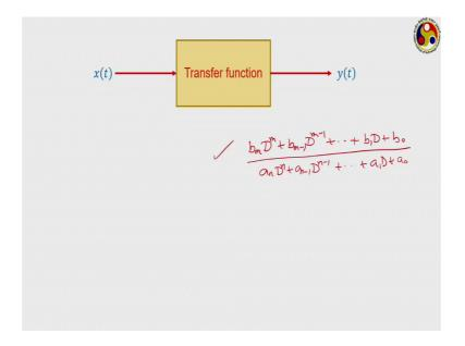
And this is what we refer as the transfer function. If I delete this entire thing, then I am sorry for this mistake, because this got superimposed with the previous one. So, in this particular example then what is your transfer function? Your transfer function is the right hand side that we wrote earlier, where we have this; these this are the numerator, and this is the denominator. This is the transfer function for this particular system.
