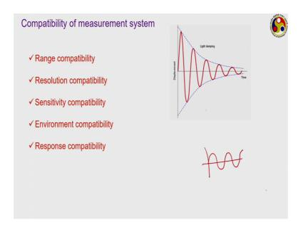
Next is the sensitivity. Sensitivity can also be important, generally we always prefer the instrument to be to have higher sensitivity that is the same change in input should cause a larger change in the output. And if the sensitivity is not sufficient or is very small, then we may not be able to get the correct output value or may not be able to note the correct output value, because on the scale the graduations may be very close to each other.
