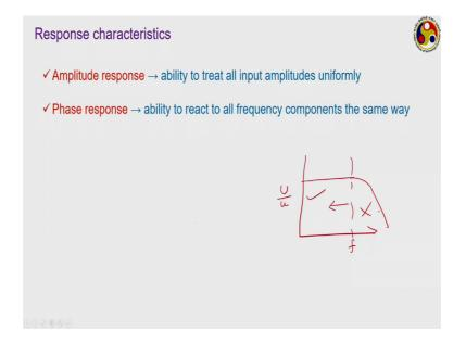
Like, suppose if we plot frequency on this axis is the frequency one axis, and this gain that is output by input on another axis, you may see that the device may have a good phase response over certain range of frequency. But a very inferior one after that that is so again we should use the device only in this particular range, but not in this range, because for this cross range the frequency response is poor.
