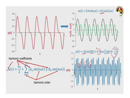
And any periodic signal can often always be represented in a form like this, like the example. The signal that we had here actually is a combination of these two signals. One is a red one, another is a green one you can clearly see their amplitudes are different.
