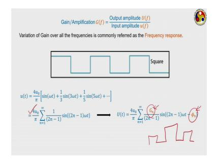
Now, as I mentioned gain or amplification is referred as the output amplitude to in fluid this ratio. Variation of again over all the frequencies commonly referred as the frequency response. Like and let us say it is a square wave, we know that the square wave is represented by a signal like this or we can sum it up over this particular form, which we have already seen in earlier slide.
