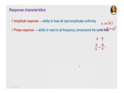
Think about two periodic signals, just we are repeating this similar kind of example. So, we have two periodic signal. One signal is having a form a sin omega t, and other signal is having a form a sin twice omega t plus some phi where phi is the corresponding phase difference.
