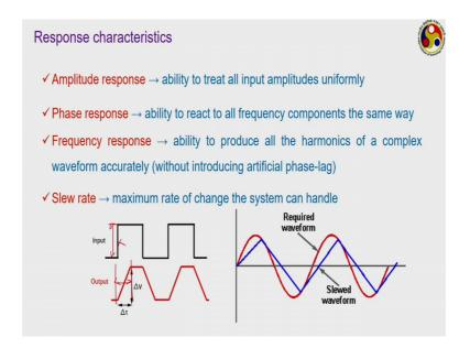
The last one is a slew rate, this is a maximum rate of change the system can handle, every system because of its own characteristic has certain rate of change that can be handled properly. Like one example, we are providing a square wave, but the system cannot handle such large change in input. So, it is showing the response that is low like this that is over this period, it is having a kind of lag.
