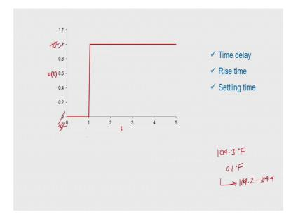
Like while measuring the body temperature, if the body temperature is say 104.3 degree Fahrenheit, then we may choose a band of something like 0.1 degree Fahrenheit that is was the time becomes restricted between 104.22 104.4, then we may say that it has raised the settling time. It has attained the settling time, it has settled in a 0.1 degree Fahrenheit band.
