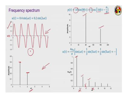
Now, as you can see that just going back to the example that we have studied. Here this signal is a combination of two sin waves, which are having amplitude is 0.4 and point when their frequencies are omega and twice of omega. Now, if we know these amplitudes and frequencies you can clearly represent this one both in terms of mathematical form and also in graphical form, and so while this remains the most common way of repressing the signal that is signal with respect to time.
