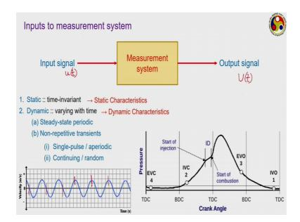
We now know from our discussion that in any measurement system, we generally have two kinds of interface. The input stage creates an interface between the physical system with your measurement device, where it collects the input signal from the physical system. Quite often that input signal is compared with some kind of standard reference to provide a transducer signal, which goes through the second stage the signal conditioning stage.
