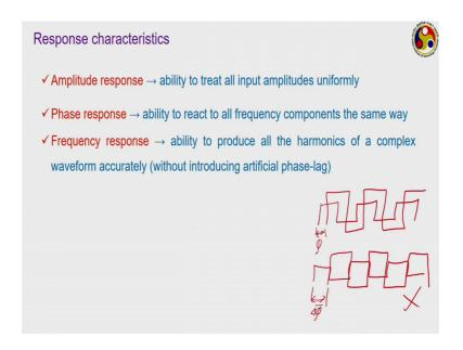
Suppose, your input signal is a square wave kind of thing. Now, if the signal is not having a proper frequency response, then it let me give you another example. Suppose, your input signal is a combination of two square waves, this is one, and the another square wave which is lagging this one by a certain distance, this is the lag.
