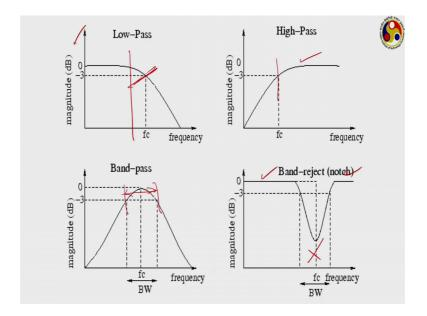
Just one example about how sometimes we can use the frequency response to our advantage that is what we have done in filters. Here this side we have the gain, and this on the (Refer Time: 58:20) of the frequency. Now, over this particular range the system is showing a constant gain. The gain keeps on changing, and after this there is a drastic drop this.
