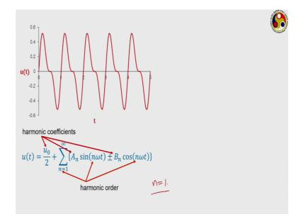
Now, look at this particular signal. This is definitely periodic signal, but it is no it looks somewhat like a sin wave also, but definitely is not a proper sin wave. Then how can we deal with such signals which are periodic in nature, but does not represent does not resemble any sin or cosine wave directly? In that case, it is possible to represent any periodic signal as a combination of sine's and cosine's who is something which is known as the Fourier transform.
