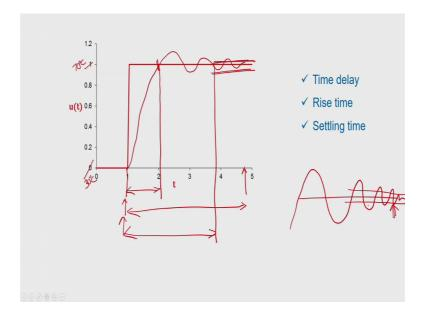
Now, that time the instrument requires to reach from its initial position to the first point, when it attains the output value, this particular time is known as settling time. We are seeing there is a significant amount of time delay between imposing the input signal, which is this is the point where imposing the input signal and you are finally getting the
