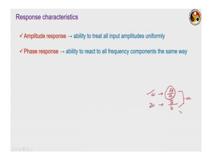
The next one in line is the phase response, it refers to the ability of the device to react to all frequency components the same way, and that means, what the example that I have just erased. For the first case, the frequency was omega for the first signal our frequency was omega, and it showed a ratio of capital A upon small a.
