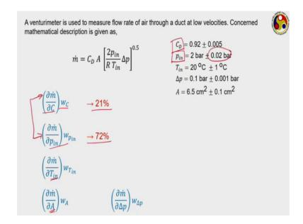
And this another problem was given for venturimeter again there are five different parameters which can five different measurements that we have to do to get the final value of mass flow through mass flow of air through the duct.
