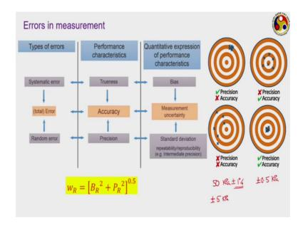
However in this full scale part is not mentioned, then the quantity of corresponding error will keep on varying with the output like when the output is 250 kilo Pascal, then it will be plus minus 1 percent of that that is corresponding error is 2.5 kilo Pascal whereas, if your output is in this 50 kilo Pascal it is 1, it is 0.1 percent of sorry it is 1 percent of that that is 0.5 kilo Pascal.
