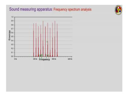
Next the frequency spectrum analysis, now from microphone or from this the circuit they talked about the sound level meter we can only get the amplitude of the power, but no information about the frequency; for which we have to go for this frequency spectrum analysis where the frequencies are plotted and the energy of the signal at different frequencies they are compared.
