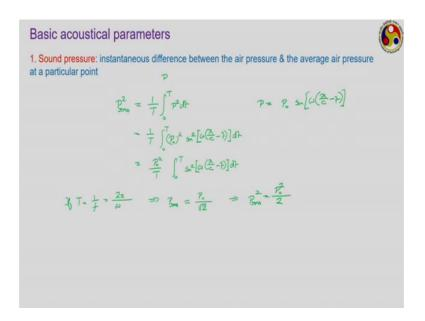
And with this let us define a few parameters which are commonly used for any kind of acoustic measurements which are the basic acoustic parameters. The first one is the sound pressure, it refers to the terms sound pressure refers to instantaneous difference between the air pressure and the average air pressure is a particular point, that is average air pressure is a before when it is not subjected to sound wave and the air pressure is the one when it is subjected to certain kind of sound wave.
