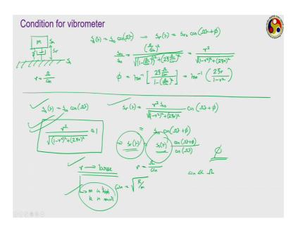
First the condition for the vibrometer, but before I directly go to the vibrometer just think about the analysis that we have done in the previous lecture where we considered a simple mass and a simple mass which is connected with some vibrating member. Say this one may be the surface where we are looking to measure the vibration. This is the mass
