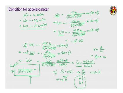
So, again we first check the imposed part. We know that the imposed displacement S s t is equal to S s naught cos of omega t. So, correspondingly imposed velocity is equal to minus omega S s naught sin omega t which you used in the previous slide for a velometer. But now, our objective is on acceleration.
