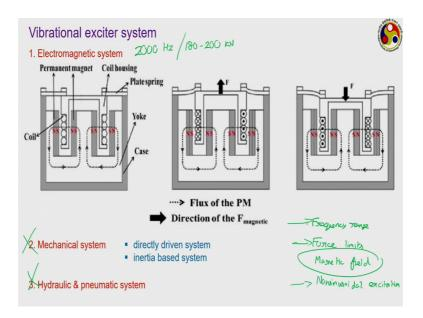
Vibration exciter systems are the systems which are used to impose vibration on certain member. Now, exciter system can be of different kinds. And depending upon the working principle, but three of them are very common. Particularly, the most popular one is the electromagnetic system.
