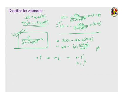
Now, we move to a velometer, for a velometer so, we again used our condition. We have our imposed displacement S s t is equal to S s naught cos. So, this is the imposed displacement. Then, imposed velocity is the time derivative of this particular thing which becomes minus omega S s o sin omega t.
