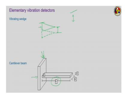
The vibrating wedge is nothing, but a triangular shaped wedge something like this which is mounted on a surface and this particular surface when it comes in contact with any vibrating member this particular surface, then this wedges keeps on vibrating and as the wedge keeps on vibrating its position keeps on changing continuously.
