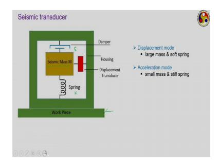
But, the most common way of doing this is use the use of seismic transducers. A seismic transducer is nothing, but a spring mass damper system here we have a large mass generally called a seismic mass given by M. There is a spring, let us say the spring is having a constant K and we are also having a damper let us say the zeta is the damping coefficient. So, this entire assembly is how in located inside a house and we are having this work piece which is the one that is undergoing oscillations.
