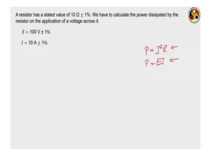
In one case I have given you a register which is a stated voltage of 10 ohm plus with an uncertainty of 1 percent. We have to calculate the power dissipated by the resistor on the application of a voltage across it. Both value and uncertainty in corresponding voltage and current are given.
