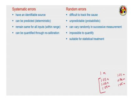
Random errors; however, are very difficult to track very difficult to identify the source of such kind of error they are very very unpredictable often leading to random change in the successive measurement like in three successive measurement we can get complete three completely different value going in three different alternate directions.
