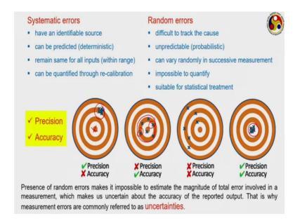
A device can be said to be precise if the random errors are very small or negligible whereas that of accuracy generally deals with the systematic errors a devices accurate means it will have very less systematic errors.
