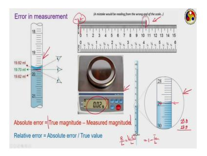
Now, some common errors; the one the picture that is shown here I am sure all of you are aware about, this is called the parallax error. Like if your objective is to get a measurement of the this particular lower elevation or sorry, the lower surface of this interface then depending upon our position of I we may get different values (Refer Time: 23:59). Its a very very common kind of error that generally quite come you know I would really miss during observation.
