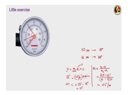
Let us take the example of a simple dial gauge a simple tire gauge I should say. So, once we connect this device to the location where you want to get the pressure measurement we get the reading in the form of rotation of this particular indicator over this particular dial. Now, let us try to identify the a few of the static characteristics of this particular tire gauge just from observation.
