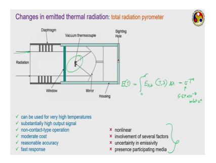
These are just some kind of common radiation measuring instruments. The first one is a total radiation pyrometer which is something like a total measurement measure overall wavelength there is no filter used emissions of all wavelengths are allowed to come.
