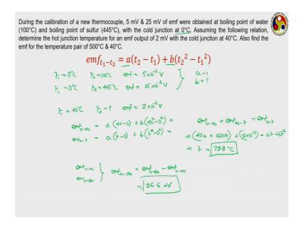
And finally, we shall be rounding off with a small problem on the use of thermocouples. During the calibration of a new thermocouple 5 milli volt and 25 milli volt of emf were obtained at boiling point of water and boiling point of sulphur, with the cold junction at 0 degree Celsius.
