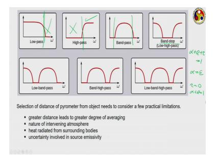
For the perp, for this purpose we generally depending on which wavelength we are interested in, we can use different kinds of filters like shown here, if our interest is low frequencies then we is low pass filter where the freq wavelength corresponding to lower
