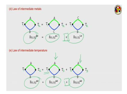
So, a fourth one very important one, Law of intermediate metals like if suppose two material A and C. Let me do these corrections, I do not know why the suffixes are missing here suppose we are using a thermocouple comprising of metal A and C and we are getting and they are maintained at temperatures T 1 and T 2 both junctions then whatever e m f we are getting that is this much.
