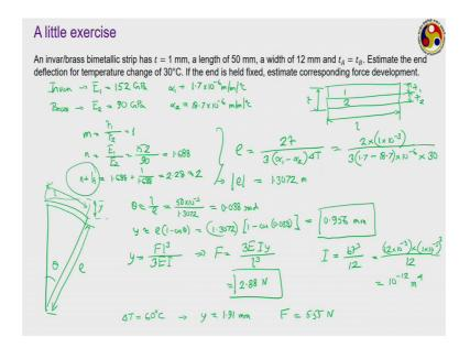
So, the value of rho is here; let us put the numbers. So, we have 2 into t, the thickness is 1 millimeter. So, 1 into 10 to the power minus; I keep on repeating always use the S I units. So, we have converted this millimeter to meter to make the calculation consistent divided by 3 into alpha 1 minus alpha 2. So, here alpha 1 is 1.7 minus 18.7 into 10 to the power minus 6 into delta T is 30.
