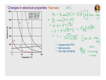
Thermistor or semiconductor based devices for and its operation is operating principle is just opposite to the RTDs. The thermistors generally had made of devices which are having negative temperature coefficient of resistance. The RTD materials generally have a positive temperature coefficient so that with increasing temperature resistance increases, but thermistors are made of semiconductor devices whose resistance decreases.
