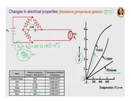
Sometimes we may like to leap calculate the corresponding coefficient of temperature rise for that purpose we have to differentiate this expression in terms of temperature which is and then we shall be dividing this divide the value of R naught. This is called the resistor temperature coefficient of resistance or just temperature coefficient.
