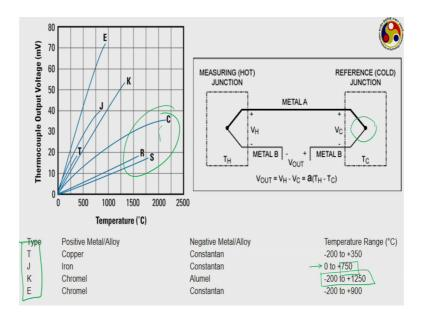
These are the response as you can see the E type thermocouple has the highest sensitivity J, K or T thermocouples also quite good sensitivity compared to this R, S or C kind of thermocouples.
