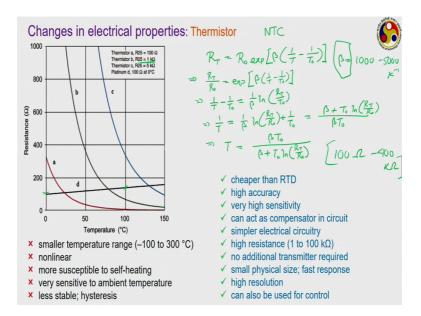
They can act as a compensator in circuit because most of the common material generally have an increase in resistance which increase in temperature, but thermistors have a decrease in resistance. So, they often can act as the compensator in common circuitry the operating circuitry or electrical circuit also becomes much smaller like they don't have any kind of lead or issue lead or error kind of issues.
