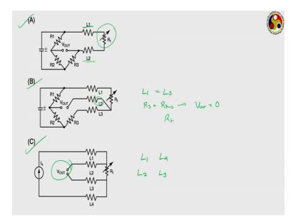
This is the one that is in early called a 2 wire configuration which is the general configuration where we are connecting the actual resistance with these two resistance L 1 and L 2.
