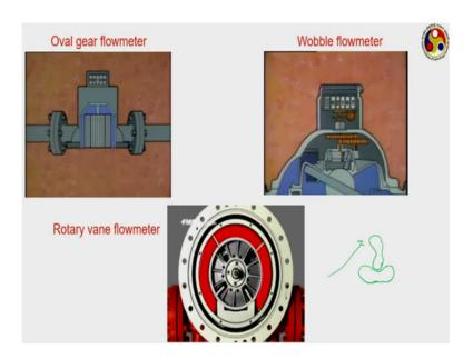
And I have a few animations for this is us for the same scenario that is oval gear flow meter. The 2 gears you can see the gears are connected to each other through the teeth. And as the fluid is flowing the gears rotate in opposite directions and allow the fluid to flow through. During each motion you can see a fixed volume of fluid is allowed to pass through a fixed volume of fluid is connect up or collected and then discharged to the to the outlet side.
