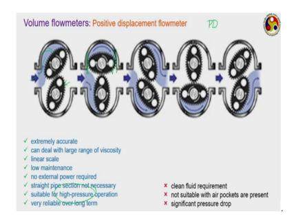
Flow meter they are extremely accurate only where there can be loss is through the small gap which maybe there left in these in between these portions general they are quite tight fit well sealed through the use of lubricating oils, but there may be small amount of slippage otherwise they are very accurate, can deal with large range of viscosities. In fact, they are more suitable for high viscosity fluid because higher the viscosity lesser is the chance of slippage through that gap.
