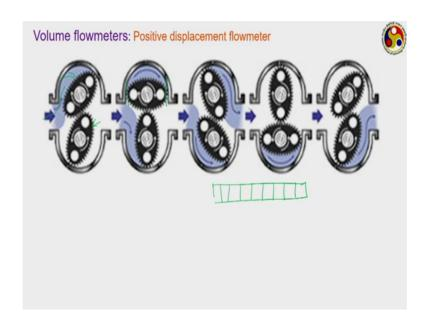
Here the idea is the in entire flow is generally divided into several small components. The components are selected such that each of them has a fixed volume then just by counting the number of components we can calculate the total volume flow rate like. Let us suppose this is the fluid volume that is flowing through.
