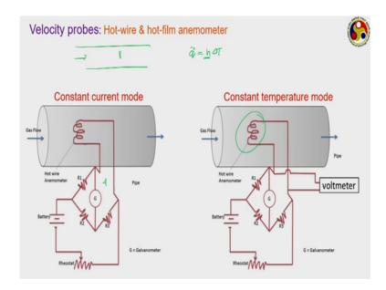
And next one a very common instrument is the anemometer, which as I shortly mention shortly back it uses the same principle as a thermal mass flow meter, but is used for velocity measurement. We can have 2 types of anemometers hot wire anemometer or hot film anemometer. The idea of anemometer is that in case of an anemometer, we generally have a if this is your flow stream.
