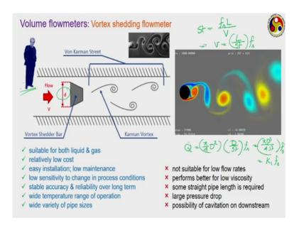
But the next one is a quite innovative one, which is called the vortex shedding flow meter. Now what do we mean by vortex shedding that is whenever we are putting a block body that is a block like this inside a flow stream, then the fluid has to find a way pass to this one that is a flow which is may be the this if we draw the streamlines which are initially just horizontal lines. They have to find a way around this one some of them or rather one of them may reaches a stagnation point.
