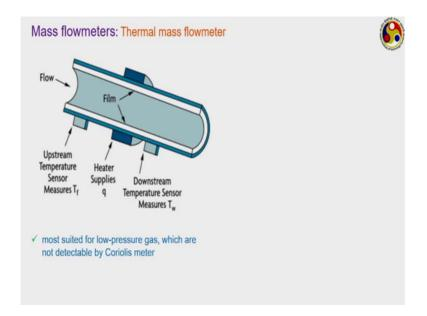
Thermal mass flow meters can have very interesting operating principle here what we are doing is that we are aligning some fluid to flow through a duct.
