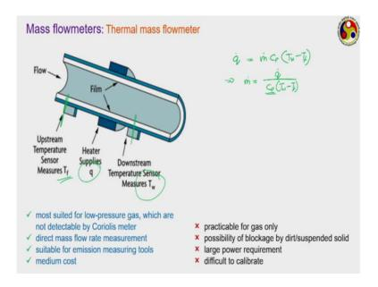
At this particular section we are measuring the temperature given by T f at this particular section we are again measuring that temperature T w and within this portion a supplying a fixed quantity of heat q. Then this rate of heat transfer q dot can be written as m dot mass flow rate into C p into the change in temperature. That is T w minus T f or I can write m dot is equal to q dot by C p into T w minus T f. Now if we can give a constant
