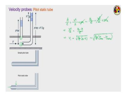
And the first one we you already know about this the pitot static tube or I should say the pitot tube. In the case of a pitot tube the configuration is shown we can have 2 piezo meters one connected on side of this tube which is going to give you the static pressure the other one connected to a inside a stagnation point inside the flow domain they were giving you a stagnation pressure.
