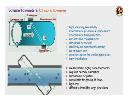
Insensitive to the pressure and temperature; so, we can easily use them for very high pressure situation very high temperature flows just like the flow of steam or in the power plant turbine or maybe the flow of hot combustion gases inside an ISO engine they can
