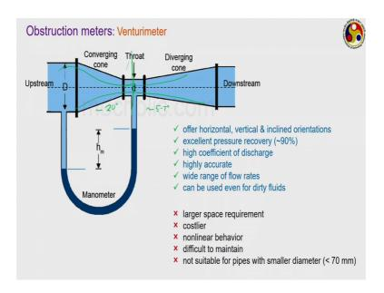
Next we move to the venturi meter, which can be visualized to be a combination of two channels. One with a converging section, other with a diverging section such that there is a common area in that throat at the throat. So, here both on upstream and downstream side, there is a smooth transition of the flow. The fluid is able to change the area quite smoothly on both upstream and downstream side.
