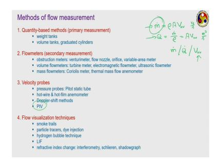
Now, the measurement of fluid flow can be done in different ways, because here not only the flow, rather whenever you are talking about the fluid flow measurement. We are also talking about the measurement of fluid velocities or maybe the mass flow rate as well and then trying to correlate the flow rate from there.
