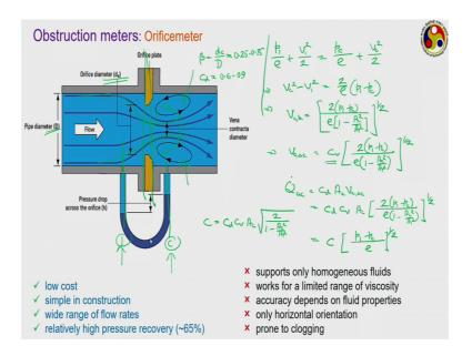
Now, there are quite a few different kinds of obstruction meters with working principle remaining very much the same like shown here. The first one the simplest one is an orifice meter. Here the idea is you have a flow channel, and in a particular section on the flow is suddenly have incorporated an orifice, just like shown here.
