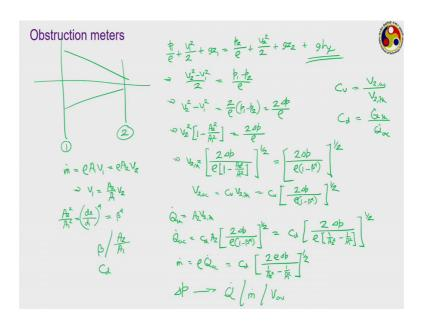
So, accordingly it becomes C two into 2 delta p by rho into 1 upon A 2 square minus 1 upon A 1 square and if you are interested in mass flow rate that is exactly, when the row comes into picture, so rho into Q dot actual. So, as rho goes in it will be the coefficient of discharge into 2 rho delta p divided by 1 by A 2 square minus 1 by A 1 square whole to the power of half or you can remain continued to be in terms of the coefficient beta or the ratio beta, yes.
