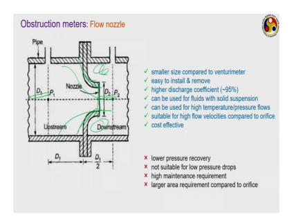
So, to eliminate that next step, we go to the flow nozzle. In case of flow nozzle, on the upstream side we provide a quite smooth change in the cross section area. From the initial pipe diameter D 1, it smoothly moves to the orifice diameter D 2 through this nozzle kind of configuration. However, at the exit it again is suddenly gets exposed to the entire cross section, so leaving for vortices formation in this particular zones.
