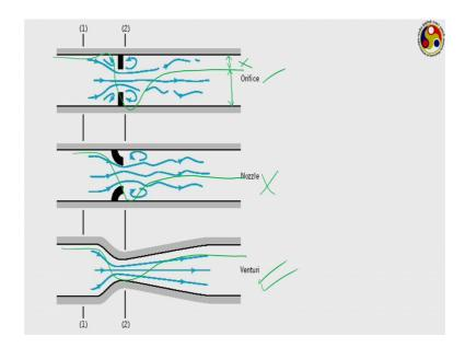
And finally as before I close in, I need to talk about the pressure recovery. In case of an orifice meter, there is a sudden change in flow direction. So, accordingly, there is the sudden drop in fluid pressure. If we follow the fluid pressure, you may find there is a slight increase the fluid pressure, then there is a drastic drop across orifice. And then it tries to recover to fall gate regain something like this.
