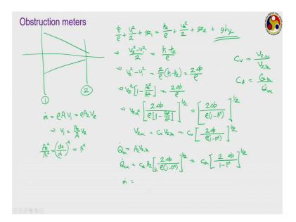
But, let us now move to our discussion on flow measuring instruments using this concept of Bernoulli's equation. And for that first we have this obstruction meters. Now, under the obstruction meter, we are talking about the measuring tools, where actually you are putting some kind of obstruction in the flow field. Thereby causing some kind of artificial pressure drop or some additional pressure drop and then measuring that pressure drop to get an idea about the flow velocity.
