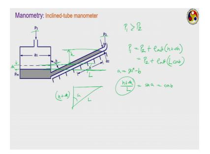
And therefore, we can go by just modifying the design itself. We can change the sensitivity of the instrument or rather increase the sensitivity of the instrument. So, I shall be quickly discussing about two of the methods. One is to use the inclined tube manometer, it is the well-type configuration or quite similar to the well-type configuration.
