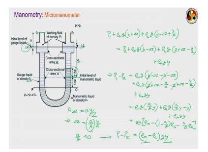
So, delta z is small a by capital A into y by 2, we can take it back here. So, P 1 minus P 2 is equal to rho w g into h minus delta z minus h minus delta z, so that corresponds to rho w plus the gauge fluid. We saw on the left hand side and we are taking from the on the right hand side we had this, this is coming plus rho m g y, so delta z goes off that is rho w g into for this was I should not have struck this out h minus delta z minus h minus little actually h goes off so 2 delta z remains.
