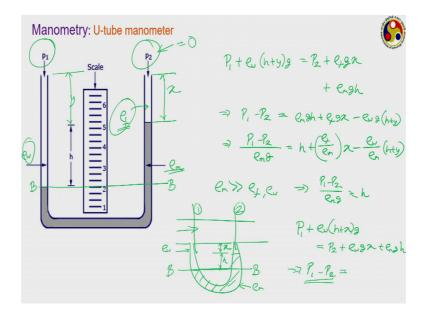
So, the next kind of manometer that we get the other variation, where we do not have a liquid pool rather we just have one tube, which is bend in the form of an U. One side of the tube or rather both the arms can be connected to different locations, we can also keep one connected to the location or you want to measure the pressure, other key being open to the atmosphere.
