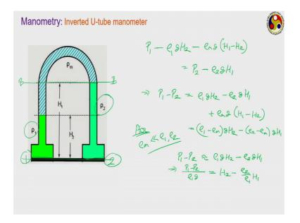
And in that situation, therefore what we do is just to invert the manometer in a configuration like this, this is called an inverted U-tube manometer. In case of a inverted U-tube manometer, let us say this is your location, where you want to measure the pressure, this is your location 1, this is your location 2.
