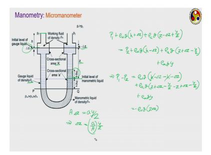
The other way of increasing the sensitivity is the use of micro manometer. In case of micro manometer, we are still using an U-tube manometer, but here both the ages or
