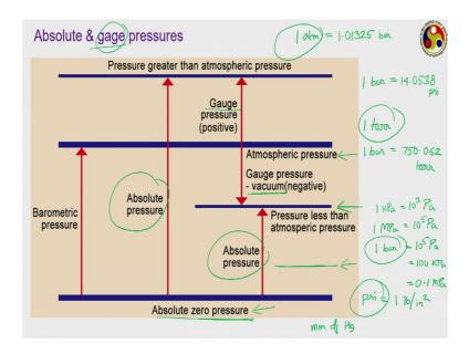
At sea level, the standard atmospheric pressure 1 atm, atm is also commonly used as an unit for pressure is given as 1.01325 bar that is slightly above 1 bar and that is the reason of having bar as such important unit of pressure. Now, one atmospheric pressure is not 1 bar, but slightly greater than this. But, this is that pressure value at sea level, these are normal atmospheric pressure.
