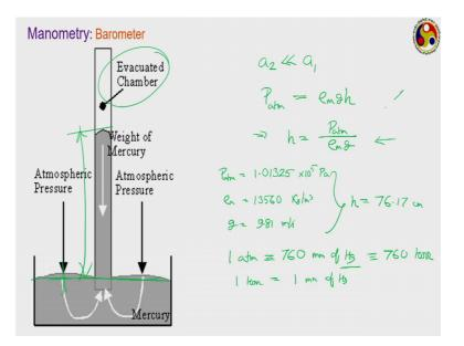
Here we have just one liquid pool which is open to atmosphere, and a small diameter liquid column cylinder, which is generally a capillary tube. And as the atmospheric pressure app gets applied on this, if we take a pressure balance at this particular location, then the atmospheric pressure which is acting at this particular point has to be balanced by this particular liquid column.
