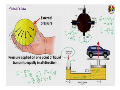
Now, that direction independency is given by the Pascal's law, which all of you have definitely learned at the school that is at a particular point on a liquid or maybe on a gas also on a fluid if we apply pressure, then force is transmitted equally in all possible direction, which essentially prove that pressure is a scalar quantity and that also has lots of applications in practice.
