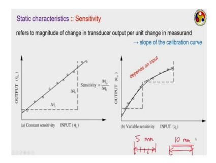
So, this in this particular case the slope does not change with the change in the input, so we call it a static constant sensitivity how we may also face situation, where the sensitive at instrument keeps on changing the input. Then it is a variable sensitivity, because it is depend on the input.
