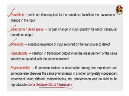
If you lesser is properties dead time refers to the minimum time required by transducer to initiate any response, like in this example itself. As now we changing the input of this period and not getting any kind of output, only after reaching here, we are getting any response from the output device.
