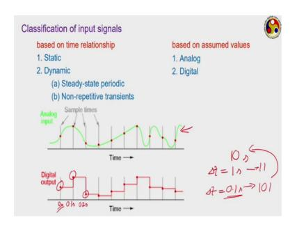
Now, the input signal the input signal can be classified primarily into two categories or we can have primarily two kinds of classification. One based upon the time relationship means, how the input signal is wearing with respect to time. And second is based upon the nature of the magnitude of the input signal. The based on time relationship we can have static or dynamic. Static refers to the input is not changing with time.
