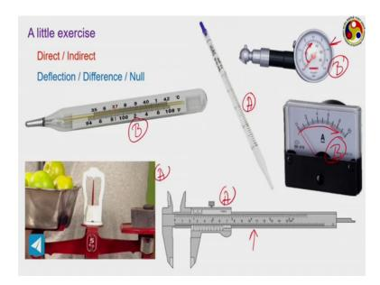
So, while the first three kind of instrument of let us say this one, this one and this one, we call them type A instrument where we are measuring exactly what we want to measure, but this is a type B instrument where we are not measuring, what we are trying to measure rather we are measuring something else and then identifying a correspondence between our objective measurement and this modified one.
