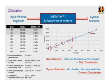
Now, we come to the stage of calibration. Any instrument has to be calibrated to start with and calibration means, the instrument will be subjected to a known magnitude at the input stage and output stage, whatever response we are getting in whatever may be the form we are going to record that and then try to identify the correspondence with your input.
