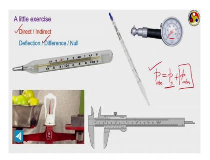
But, if our interest is to know the absolute pressure, then you have to the final pressure value which is the absolute pressure that your looking for that will be the gauge pressure returned by this gauge plus the atmospheric pressure, which you have to collect from some other source (Refer Time: 10:02) something that means, here we do have a reference.
