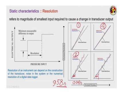
Next is resolution very very important for an instrument. It refers to the smallest input required to cause a change in the transducer output. Smallest change in input required to cause a change in the transducer output, this is different from sensitivity. Here like we are causing initially your system is having a pressure value of this and corresponding output is this.
