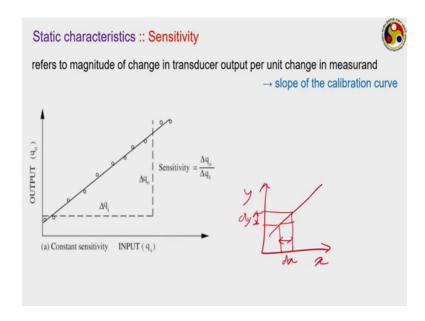
Let us discuss about a few properties of the static the characteristics, which an instrument must have. The first one and the most important probably is sensitivity. Sensitivity refers to the magnitude of change in a transducer output per unit change in the measurand means, it gives you the slope of the calibration curve.
