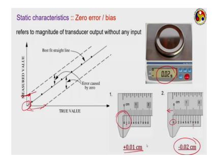
Next is zero bias, it refers to the magnitude of the transducer output when you are not given any input at all. There may be several situation like ideally in case of ratio measurement particularly, we want the output to be 0, when there is no input. But, sometimes your instrument itself, we have some error inside and it starts the reading from some this particular point itself. You must have seen such situations with us weighing scales.
