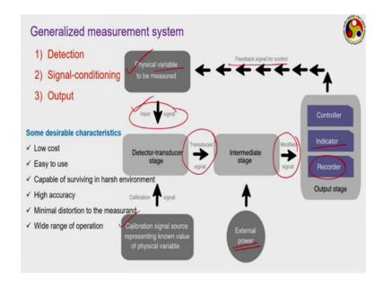
Next move to the general structure of the measurement system. So, in a measurement system all the components whatever simple it may be, whatever complicated it maybe, we can generally identify three different blocks; one detection block or input block, next is the signal-conditioning block and next is the output block.
