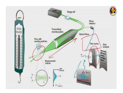
Next we talk about a few examples again. First we have a spring balance; you know spring balance is used to measure the weight of something. So, we put the measure and somewhere here, and that causes that corresponding gravitational force causes a deflection of the spring, which is inside the inside the body and the deflection of the spring causes a change the position of this indicator.
