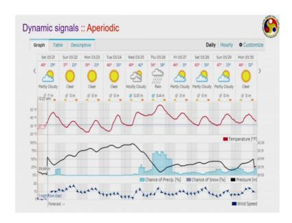
Aperiodic like the variation of temperature over a period of day or over a much longer duration the any kind of whether data that is only the example of a dynamic signal, which is not periodic in nature at all. And in several measurement situations, we face with a period dynamic signals.
