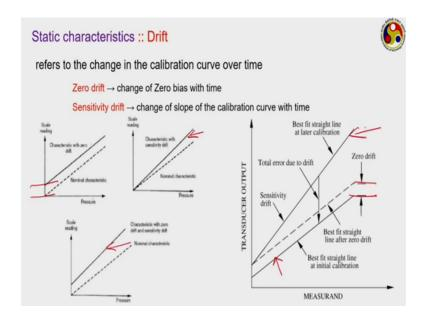
The final characteristic that you would like to talk about, this refers to the change in the calibration curve over a period of time. Now, once you have calibrated the instrument because of different kinds of ageing problem, warranty or certain damage the calibration may get shifted.
