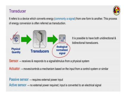
But, this is another example were some physical quantity in a transducer getting converted to an analogues signal, but here also we are measuring temperature. But, your input temperature is temperature sorry input signal is temperature and output signal is some electrical quantity like what happens in case of a thermocouple.
