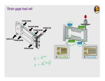
I shall briefly be touching upon on another one that is on strain gauge load cells. We have already had extensive discussion on the strain gauges; strain gauge load cell just uses a
