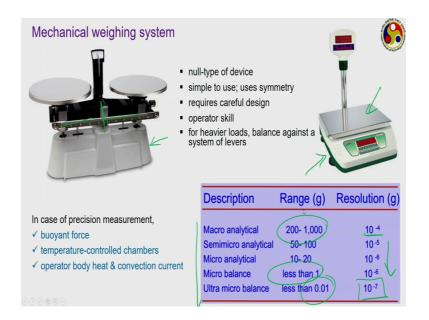
Now, the first one that we have in line is the mechanical weighing system. I am sure each of you have seen this particular thing, this is what we commonly use for measurement of mass. But, actually does it provide the measurement of mass, actually what it measures is the force. Because, whenever you are putting, something say on this particular arm, we are trying to balance that by putting a counterweight on this other arm.
