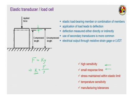
Next type of device that we have elastic transducers or load cells. Load cells are devices quite similar to the one that we have seen in case of displacing measurement. Here we have an elastic member, when subject to some kind of force, it suffers some kind of deformation. So, there is a change in length, and also change in the cross section area.
