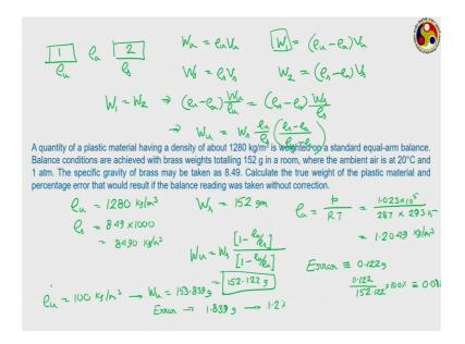
Let us quickly check, how the presence of buoyancy can affect. While it is very difficult to element the convection currents and the effect of temperature, but the with simple calculation we can eliminate that buoyancy part. Like suppose, we are trying to measure the mass of a body, say this is our body for which you want to measure the mass, this is 1 and this is a one, this is the counter weight that is 2.
