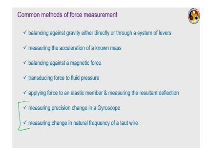
Now, the common methods of force measurement, there are several ways we can measure force. And you have to remember that always we are actually trying to play around with a mass and corresponding acceleration to get the magnitude of force. And now what kind of acceleration we are talking about accordingly, the measurement principle may vary.
