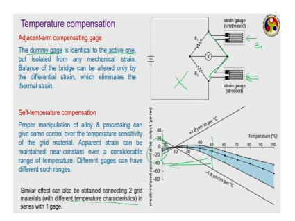
Now, we move on to the next topic, which is the temperature compensation. Now, you always know that the temperature of any kind of resistance is strongly affected or I should say the value of the resistance of any register is strongly affected by the temperature. Generally, the nominal value that are specified with a register corresponds to any particular reference temperature. And whenever the temperature varies from that position, there is a change in the resistance.
