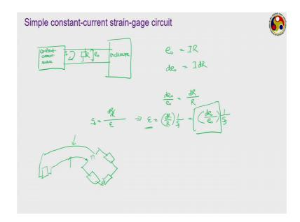
Now, let us move forward to the third kind of electrical circuit that we quite often use in conjunction with the strain gages, it is the simple constant-current strain-gage circuit. So, what we have here? Here we have a constant current source which is connected to some kind of voltage measuring instrument, which can be an oscilloscope.
