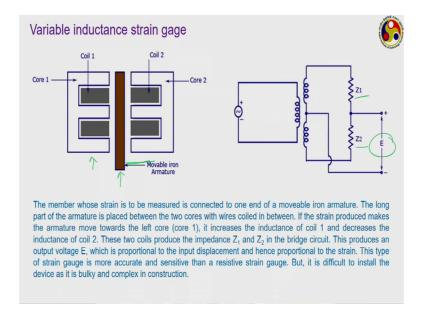
Similar to the displacement measurement like resistive instrument, you can also have inductance and capacitance base instrument. And that is why this is a very brief introduction about the variable inductance strain gage. Here we have a moving an iron armature, and the instrument for which we want to measure the strain of the specimen that is connected with this armature.
