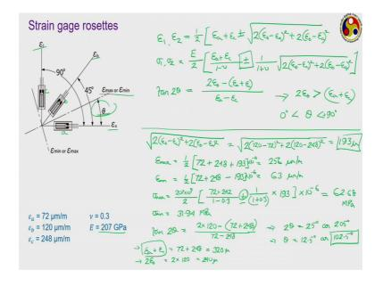
Rosettes primary combine of primary is a combination of three different parameters like shown here, this is just one particular rosette, which is very commonly called the rectangular rosette. Now, in this particular rosette, you can see there are three gages and they are placed 90 degree apart from each other.
