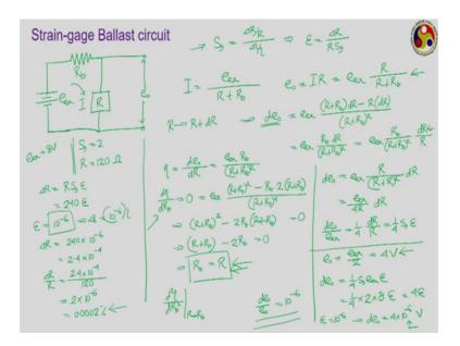
The first kind of electrical circuit that we use in connection with strain gauge is something known as a Ballast circuit a ballast circuit is somewhat similar to a potentiometer application very simple we have a voltage source something like this we have a resistance connected with this and this is your strain gauge. Let us say this voltage is e e x, R is the gauge resistance and R b is this ballast resistor and then across this you will be measuring this output voltage e naught.
