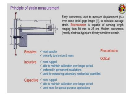
Now, the principle of strain measurement; the there are several ways we can measure strain. In early day instruments generally they used to measure the displacement delta 1 over a certain length and then the displacements were used to be divided by the actual length thereby getting the value of the strain. Extensometer is one of the earlier instruments where this displacement delta 1 used to be measured actually modified form of this one is still in use in certain applications.
