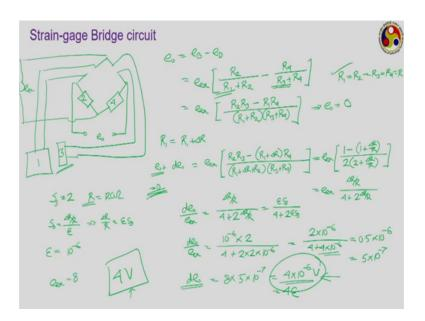
I think the initial value we calculated as a something like 4 volt. So, with respect to 4 volt output voltage initially we already have a 4 volt value at the output. Assuming a voltage measuring instrument which is having infinite resistance you are already measuring a voltage of 4 volt and in that 4 volt now you are trying to measure a change of 4 into 10 to the power minus 6 volt which is extremely difficult.
