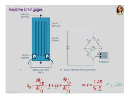
This is how a resistive strain gauge may look like. Some resistive element generally etched to a metal foil with a proper backing material and depend and they are resistive strain gauges are generally fixed with the specimen. So, once the specimen goes to some kind of deformation they are able to directly sense that and corresponding change in resistivity or resistance I should say is generally leads to a change in some kind of
