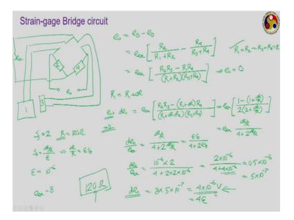
So, here situation is this 1 and 3 are cave vacant, 2 and 4 will be the normal bridge resistances. So, this is your 2, this is your 4, the normal bridge resistances they will be connected to the output voltage measuring instrument which is giving e naught. And, you also have the supply voltage at these two points which I am finding some difficulty to draw this say, ok. So, over here you have this e e x.
