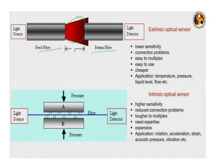
The other intrinsic where the light never goes outside rather during its passage through the device itself there is some modification in its properties. So, this second one is intrinsic. Extrinsic one generally has a lower sensitivity and leads to connection problems, but they are very easy to use we can easily go for multiplexing and they are cheaper whereas, intrinsic devices have much higher sensitivity and much lesser connection problem.
