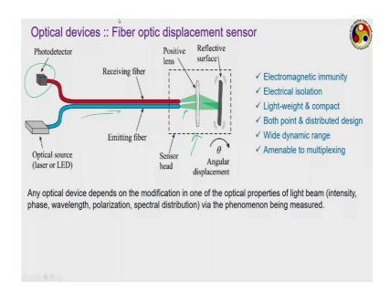
Optical devices are very common for measurement of several kinds of parameters pressure, temperature, flow, and displacement and motion are also exception. The idea particularly with the there are several kind of optical devices.
