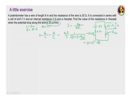
We have our 20 ohm resistance for the register plus 2 ohm internal resistance plus this R rh. This thing should be equal to that 20 micro volt per millimeter or if we can write in terms x into 20 into 10 to the power minus 3 volt per meter. So, from this the value of e x is given to be equal to 2 volt, capital is given to be 20 ohm from there you can easily identify the value of this R rh.
