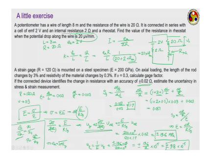
Let us now try to solve something for the strain gauge. There is a strain gauge that we have learned in the previous class. Let us try to solve the problem on that. So, quite straightforward problem is given here for the strain gauge we are having a resistance of 120 ohm then it is mounted on a specimen and the specimens is having Young's modulus of 200 Giga Pascal.
