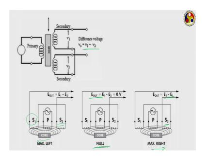
However, in most commonly we do not use the voltages that way do not use the secondary windings that way rather what we do is referred to as the series of post-secondary. The series opposing secondary refers to this just look at this diagram here the opposite ends of the two secondary coils are connected with each other there by your reference voltage V 1 and V 2 sorry the output voltage V 1 and V 2 will always be opposite to each other thereby giving v naught equal to V 1 minus V 2.
