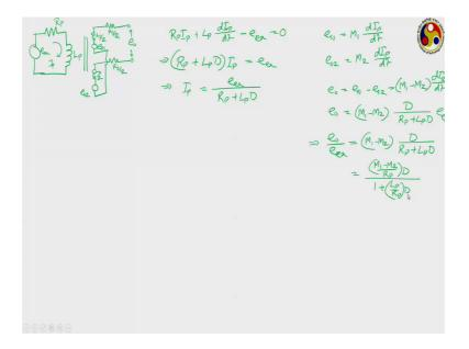
So, this is your primary side source the resistance of the primary circuit and the inductance of the primary circuit. So, this resistance let us say R primary this is L primary and this is your source say E excitation. So, a current I p will be flowing through this and this is the core and.
