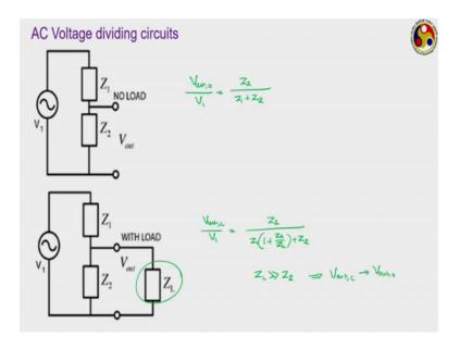
This is for DC voltage division we can have similar AC voltage division circuit just the way we have created the (Refer Time: 18:54) bridge or corresponding AC bridge circuits in last class. Just the same thing we can do just replace all the resistances with
