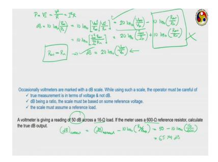
Now, for a pure resistance we know that P is equal to V into I or we can write this one as in 2 ways we can write this one as V square upon R or we can write this one as I square R. Now if we want to write this on in terms of decibel values there are 2 way we can write we know that decibel is 10 log 10 P out by P in.
