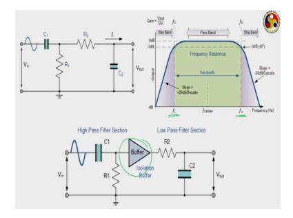
Then we have a band pass version where we have 2 cut off or critical frequencies 1 f L other f H, anything below f L or above f H are not allowed to go through. But frequencies in between are allowed to pass and sometimes we put an isolation buffer in this, is an example of an active filter which we are not going to discuss any further, where along with the band pass option we are getting the amplification of the signal as well.
