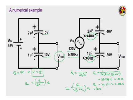
This is a numerical example of the same, here we have couple of capacitors they are connected in series and we have to measure the output voltage which is across this second capacitor of 1 microfarad versatile and input voltage is DC 1 just 15 volt. Now, for a capacitor we know that the charge across the capacitor Q is equal to V into C. So, applying the same principle or we can say for a given value of Q V is inversely proportional to C.
