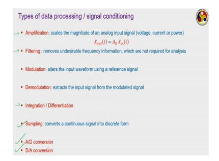
Now let us quickly move to the data processing or signal conditioning, using this analog instruments or even in case of digital instruments also we can modify the processed data into some form which is suitable for us and for that we may have to go for several kinds of data processing.
