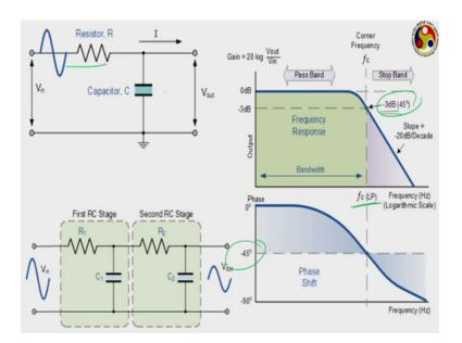
This is the one that we have just analyzed this is actually a low pass filter. The corresponding representation you will be getting like this, this is the value of f c till this f c you can find there is only minus 3 dB reduction in this and it does not allow anything to pass beyond that value of f c.
