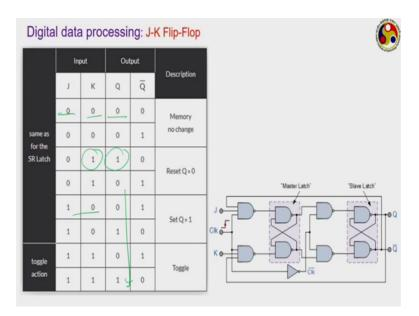
That is why people go for JK flip flops, in JK flip flop we have removed that option here we can remove that disadvantage here we can still have 0 0 kind of inputs so that you can give 0. When both are 0 there is no change in the memory output, however as soon as 1 becomes 1 there is a change and it does not change with resetting the Q to 0 and whenever Q is set back to 1 then you can see there is a change here and subsequently it keeps on changing.
