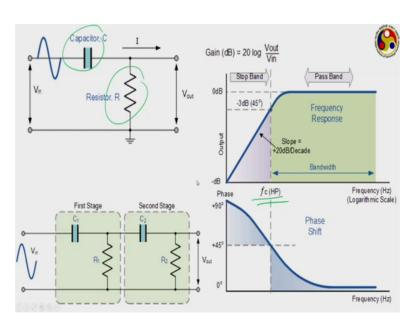
If we change this capacitor first in the line resistor in the parallel circuit we have a high pass filter, everything below this f c they are stopped and the frequency after that are allowed here also you can have such combinations and when you combine these high pass and low pass filters just like this.
