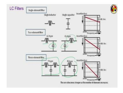
Earlier we had RC filters similarly we can have LC filters or R L filters as well, LC filters you can see there is a combination of an inductance and the capacitance or capacitance first inductance second, we can have multiple such kind of T or n kind of see a circuits as well, each one has its own way of operation.
