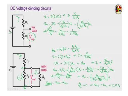
Now, let us move to another circuit which is known as the DC voltage dividing circuit. The voltage dividing circuit is nothing, but converting the output or scaling the output to a form as per our requirement. Just look at the circuit that is shown here. Here we have a voltage source V 1 and there are 2 resistances connected in series R 1 and R 2, then V out if the voltage output across R 2 is given as V out then we have to calculate the relation between this V out and V 1.
