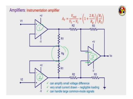
And there is another one that is called Instrumentation amplifier which actually combines 3 Op Amps, this is number 1 this is number 2 and this is number 3 1 input is supplied to the one amplifier 1 and second input supplied to amplifier 2 and both of them are connected through this ground resistors. And then the output obtained from both these Op Amps are connected to this third amplifier this one acting as the non inverting one this one acting as the inverting one.
