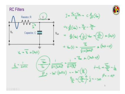
Filters can be formed by suitable combination of resistors capacitors and inductors and RC filter refers to combination of resistor and capacitor, just look at the one that we have. Here the input signal is directly supplied to the resistor and the capacitor is connected in parallel.
