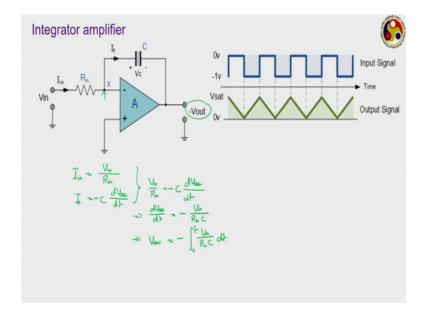
Just the opposite of this it is a integrated circuit, where is the resistance in the male line and capacitor in the bypass line to this amplifier. So, again here a voltage at the point x is equal to 0 and I in an I f are equal to each other. So, your I in will be equal to V in upon R in and I f will be equal to C into dv out dt or minus because there is a minus sign here.
