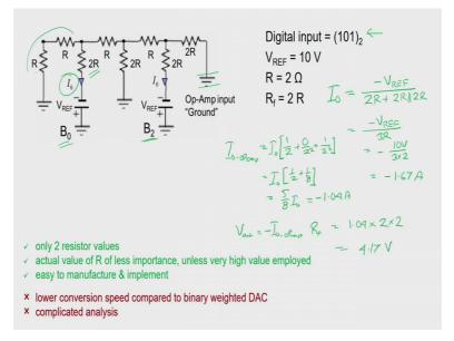
This is an example of dealing with here we are dealing with talking about a 2 bit resistor, this is the least significant bit this is the most significant bit and your input current digital input is 1 o 1 that is the most both most significant and least significant bits are set to 1 and a intermediate one is 0 the reference voltage is 10 volt here R is given to be 2 ohm and R f is said to be 2 R. Then how can we calculate the value of this current first.
