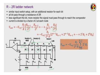
So, the next one that we have is called R-2R ladder network. So, in this case here each of your bits here your switching setup is quite similar, but we have an additional resistor for each bit. Like if you see each of these bits, this is the most significant bit this is connected with the resistor of 2R. So, all bit passed to this resistance of 2 R and then in between these 2 connection there is this resistor R, this additional resistor.
