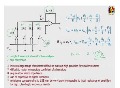
So, the biggest advantage of the structure is it is a very simple easy to understand structure it is an economical construction from design point of view and also easy to analyze and quite fast conversion. Because all of them are working parallel, so, it is very fast, but it involves a large number of resistors.
