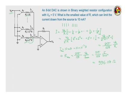
Let us solve one problem on this, here we are our problem corresponds to an 8-bit DAC here just shown here, this is the least significant bit having resistor R naught it is the most significant one having resistor R.
