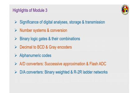
So, we started with defining the significance of digital analysis, storage and transmission over corresponding analogue counterpart then we talked about the number systems conversion from one system to the other Particularly conversion from decimal to others and from other system to decimal and from there we established how I binary is so important compared to the other systems. Then we talked about the binary logic gates, their combination to give different kind of conversion of binary digits.
