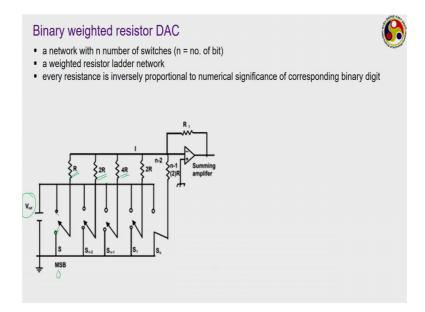
The first one is called the binary weighted resistor. In case of a binary weighted resistor, we have a series of resistors each connected to 1 bit of the binary input; that means, if there are have you are having n number of binary sorry if you are instrument is of n bits, then we are also going to have n number of resistors.
