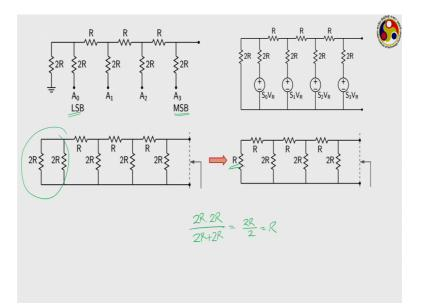
Let us take this circuit where we have just 4 bits, this is a most significant one, this is the least significant one. So, we have to keep on reducing the circuit to smaller case, this circuit can be thought to be equivalent to this where all this s naught S 1 S 2 and S 3 refers to the refers to the value of the concerned bit like S naught refers to the value 0 or 1 which occupies the least significant bit.
