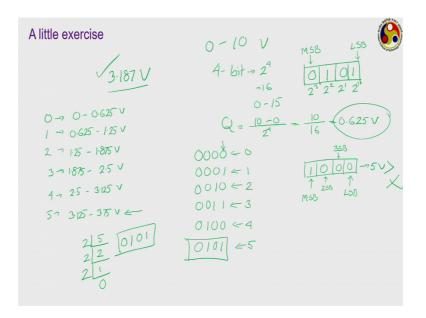
Now the when the process conversion process starts, resistor will convert the value of MSB to 1 or set it to 1, then 1 triple naught corresponding to 1 triple naught. What should be the value? The corresponding value is 5 volt. Now this is greater than this 3.187. So, this is not possible. So, this was back to 0.
