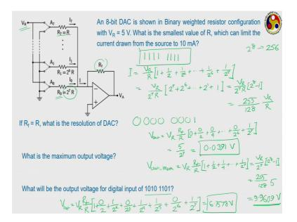
And it should corresponds to which input? It should correspond to the input of all 0's. So, this is going to give you an output of 0 volt. Now if we change this by the smallest possible amount that is change by 1, then how much is the change that your going, that is going to take place that should be your resolution.
