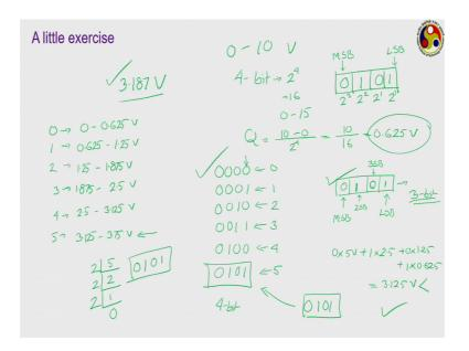
Now go to the least significant one, set this to 1; then what is the value corresponding to this? The output voltage like corresponding this binary representation corresponding digital to analogue converter will give you 0 into 5 volt plus 1 into 2.5 volt plus 0 into 1.25 volt and finally, 1 into 0.625 volt which should be 3.125 2.5 plus 0.625 is 3.125 and this is coming to be less than 3.187.
