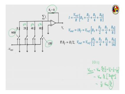
Let us take the example of this particular resistor. In this particular resistor we are dealing with a 4 bit converter. So, 4 bit means first one you have a resistor R, second one
