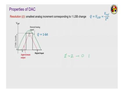
So, the it is always desirable to have higher resolution like any measurement device. We always want higher resolution; that means, with a smallest possible change in the input, we want larger change in the output; that is what the basic definition resolution is and the same is applicable here also. When you have larger resolution we always prefer to go for that device like just see this example. Here our analogue desirable analogue signal is
