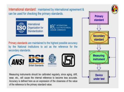
Now, there can be several kinds of standard primary secondary and also measuring or lab based standards whenever we are comparing a device for as whenever we are performing the measurement based upon the standard for measuring instrument. Then that is a secondary kind of measurement same for secondary standard, but only when we are able to compare with the primary standard we are getting much more accurate measurement.
