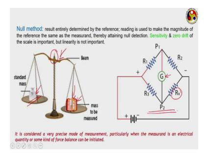
The next one is null, null method where entirely the measurement is based upon reference the best example can be such kind of weighing balance here we put the put the measurand on one side here. And on the other side we keep on adding standard mass and we keep on waiting till the indicator which may be somewhere here which shows a 0 value a null value. That means, whatever deflection of the indicator has been caused his measurand that has been negated by the standard mass.
