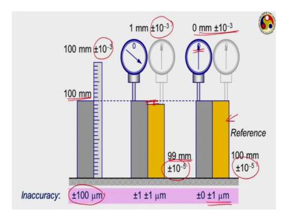
An example here we are trying to measure the length of a bar which is supposed to be 100 mm, in case of first case we are taking it in contact with a scale. And the deflection
