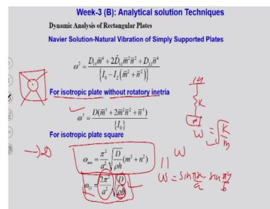
The next for the case of isotropic plate without rotatory inertia it leads to like this. If you say the plate is square, then it reduced to like this. If you say the lowest one m = 1, n = 1 then it gives you next, twice of this. So the first frequency of an isotropic plate is related like this 2 pi square plate a square under root d/rho h. If you remember for the case of a spring mass system under root K/M.
