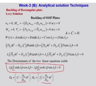
Applying those conditions, you will get these 2 set of equations. Now the set of equations the trivial solution is that B = D = 0, B or D both are 0. If A and C is already 0, if you say that this solution is, one solution is that B and D = 0 then there is no buckling, no load, nothing, no function. So non trivial solution for such cases before proceeding further you may hear about that let us say 2 x 2 matrix x1 and x2 and righthand side is 00.
