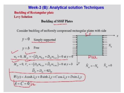
So now you are going to solve a plate which may have y = 0 simply supported and y = b2 free. So when simply supported boundary condition w must be 0 and moment along y direction must be 0. For the free case moment and vy has to be 0. So the solution is written in this form for a particular case then if you substitute that when y is 0, w is 0 and y is 0 moment is 0. So from that you will get A and C constants are 0. Now the next one y = 0, my moment is 0 and shear force is 0.
