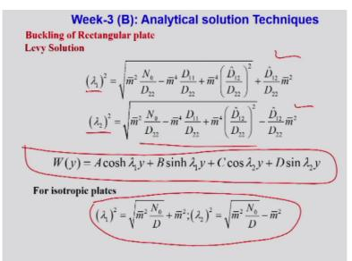
So basically you will have four roots lambda 1 square, lambda 2 square like this. So if that condition satisfies, so you can write a solution like this based on the roots thus I have already explained for the bending case, if my roots are complex, real or linearly dependent then we can write the solutions. So for the case of isotropic D11 is D, D here 2 is D so this lambda 1 square, lambda 2 square reduces to like this.
