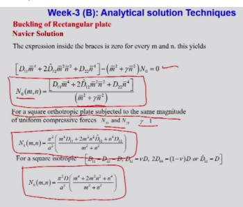
So If you are putting equal to 0, n0 becomes D11, this term divided by Mn square + gamma and bar square. So this is your buckling load, but you do not know whether it is a critical lowest buckling load or not. So this term that value of mn and the value of D1, D2, D22. Based on that only if you substitute those values and evaluate for every m and n and you find which one is the lowest that will be the first critical buckling load that first lowest.
