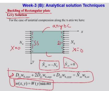
Buckling of rectangular plate for Levy type boundary conditions. So we have solved for the Navier case it looks very easy, but for the case of Levy it is not so easy. So first of all let us
