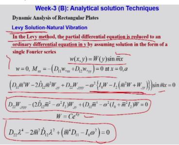
Now again for Levy type, so I am discussing this I think third time, first for the bending case, second time for the buckling case and third for the last is for vibration case. So Levy method converts a partial differential equation into an ordinary differential equation by assuming it to just simply supported. In Kantorovich you are doing or assuming a solution in ny and converting a partial differential equation into an ordinary ny.
