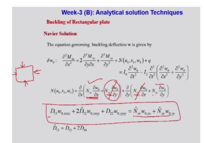
Now come to our course topic that buckling of the rectangular plate, I think most of the undergraduate students are aware about the buckling of beams, what is that buckling of beams. When you are saying buckling, basically buckling of columns not even aware about the buckling of beams, they are not just when there is a column like this and if you apply a load axially compressive load and you can get some critical buckling load.
