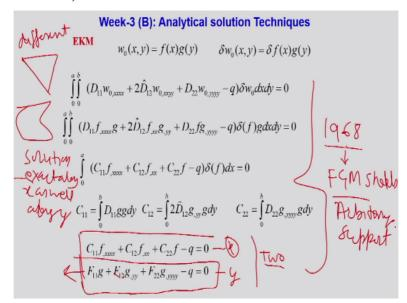
So in this equation if you substitute this values fx and ds, so where w0 is the function of derivative along x-axis. So you will get fs derivative for g remains as it is, here mixed derivative, so g double derivative y, fx double derivative y. Similarly, here w derivative y g 4 times of derivative by and del w not will be del f and gy. So here written like this, so you see del f and gdxdy = 0.
