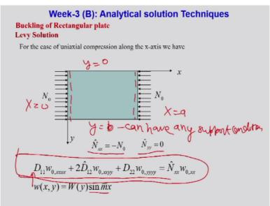
Now you talk about Levy solution which is like you have seen for the case of bending Levy solution was okay, slightly complicated not much complex like you get ordinary differential equation of fourth order, now you are solving based on the roots you can get the solution and applying the boundary condition you can solve that, but here when we say Levy solution 2 opposite edges must be simply supported.
