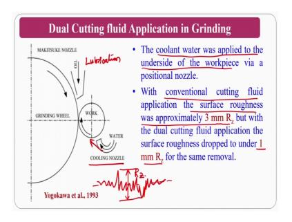
So, dual cutting fluid application as I said one side normally the people can apply water type of cutting fluid, because the temperature generation is very high. On another side you can use the oil oriented, because you need the lubrication. Whenever you are using the oil that is you are using for the lubrication and here you are using for the cooling
