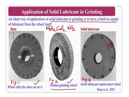
Application of solid lubricants people also uses solid lubricants, solid lubricants is nothing, but using the nano powders or micro powders of MoS 2 (Refer Time: 17:35) disulphide CaF 2 calcium difluoride and some people also uses tungsten disulphide WS 2 these are the three solid lubricants. So, ideal way of application of solid lubricant in the grinding is to have a built in supply, that is you just make the slots and you use the lubricants ok.
