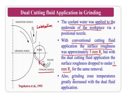
So, also grinding zone temperatures are greatly decreased with the dual cutting fluid; that means, that the author has used dual one oil another one is water, and the thing is that the temperatures also came down. So, if the temperatures are coming down what will happen you will get the good surface metallurgy.
