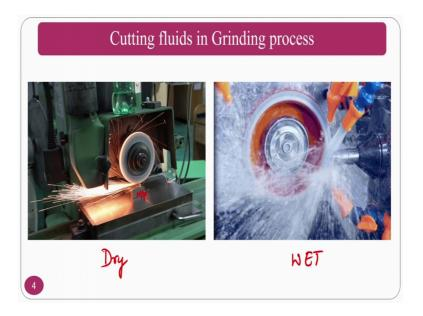
We have seen if you are not using cutting fluids the spark will come, if this is called a dry grinding and this is called wet grinding ok. If you use the cutting fluid, this will be like. If you do not use what will happen surface morphology surface metallurgical aspects of the work piece will go down. This is my work piece and which is held by the magnetic check of the grinding bet ok.
