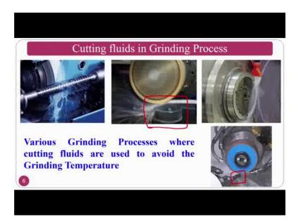
So, various grinding process where the cutting fluids are used to avoid the grinding temperatures is nothing but, you can see here the some of the grindings cylindrical grinding is there, then the lens polishing; you can see here, the lenses are grinding here.
