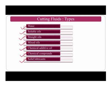
Cutting fluid types normally water based soluble oils, straight oils, mixed oils, chemical additives, chemical compounds and solid lubricants many more varieties are there. Some are, nowadays people are talking about echo friendly cutting fluids and other cutting fluids ok.
