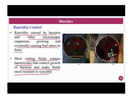
Biocides, biocides are rancidity controllers. What will happen rancidity is, rancidity is caused by the bacteria and other microscopic organisms growing eventually causing the bad odour to form; that means, that this is the grease normally cutting fluids greases these are all or the common cooling as well as lubricating agents. Since we are talking about grinding process, lubricating should be a primary concern for thus lubricating, the grease is one of the better lubricating medium.
