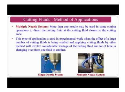
Another one which you can use is a multiple nozzle system in a milling process are this is the another since the milling and these are also comes under the multi point cutting tool processes this is also explained ok. So, if you want more details about this particular course or cutting fluids, you can refer to one of my course is introduction to machining and machining fluids, which I have previously taught on MOOCs course.
