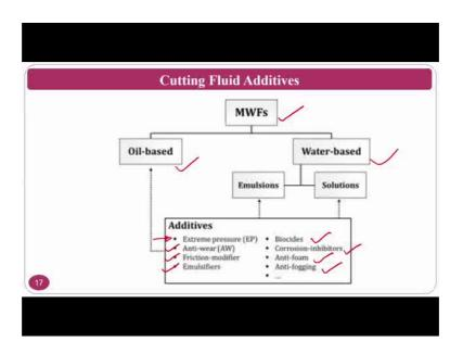
So, cutting fluid additives, the cutting fluid additives will be like metal working fluids normally it is common name, there are oil based and water based. So, if you see oil based or emulsions or the solutions, where you will have a extreme pressure additives, anti-wear additives, friction modifiers, emulsifiers, biocides, corrosion inhibiters, anti-foaming agents, anti-fogging agents, many many are there among which some are important which we will see in the upcoming slides.
