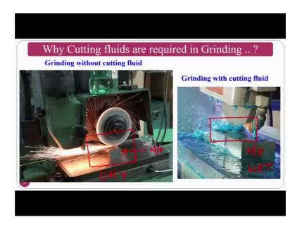
This is the work piece as you might have seen similar setup in the previous classes. So, if you are not going to use what is happening here, you see that machining region completely there is a fire type of spark is coming. So, because of this spark that temperature of the grinding wheel goes up, but since it is a non-conducting, so there is would not be problem for the grinding wheel, but the problem is the burning of the work piece.
