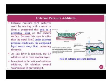
The second one is extreme pressure additives. The extreme pressure additives work by reacting with a metal to form a compound that act as a protective layer on the surface ok. So, under this extreme pressure conditions, this compound layer wears away the first that means, that these are some type of chemicals, which reacts with a work piece assume that the grinding process is going on whenever you are sending a extreme pressure additives, this will go and form a layer on the work piece ok.
