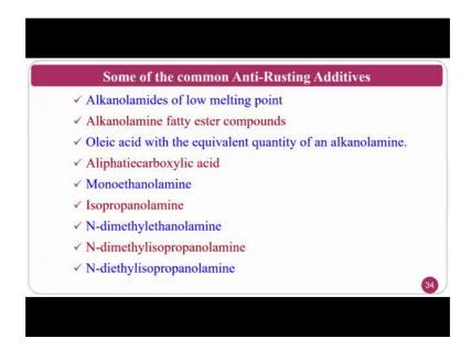
So, some of the common anti rusting additives we have seen in the previous slide alkanolamides of low melting point, alkanolamine fatty ester compounds, monoethanolamine, isopropanolamine, these are the names of the anti rusting additives that are used commonly in the cutting fluids or in other applications ok.
