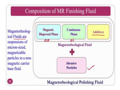
So, the first one magnetic dispersed phase you are going to use CIP particles, carbonyl iron particles; that means, that these are the ones that will form a chain from the North Pole to South Pole. So, continuous phase normally you will use suitable oils like silicone oil, grease depend on your viscosity and other things. And you will use additives whereas, I mentioned when I was teaching that MR fluid this can be as many as it used as possible depend on the functions of those additives.
