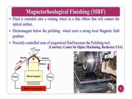
As I said this is the combination of MRF process as well as abrasive flow finishing process just we will see the glimpse, this will also brush up for your chemo mechanical magnetorheological finishing also. This is how the magnetorheological setups looks like, fluid is the excluded to the rotating wheel in a thin ribbon type of structure and whenever it is exposed to the magnetic field it will form a thin rubber otherwise it is a fluid in nature.
