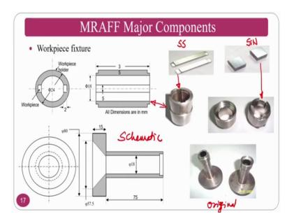
You can see the workpiece fixture where the workpieces can be housed and at the same time these are the schematic and this is the original how it looks like. So, at the same time you can see the workpieces you can have varieties of work pieces, if you see this fixture and this fixture the schematic and this one and corresponding workpieces that you can house in is this type of work pieces. If at all you are to hold this one you have to go for this type of fixtures.
