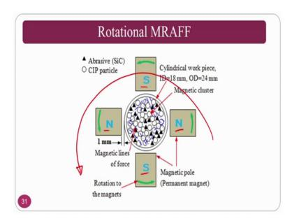
As you can see here North Pole and North Pole, South Pole and South Pole is there and these are given rotary motion, these are given rotary motions so that the finishing will be proper.
