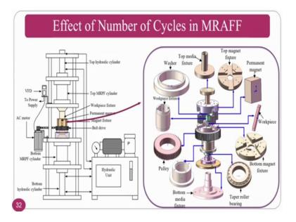
You can see the anatomy version of the fixture, so the change here is only the rotary motion is given to the magnetic field. The magnetic field that here is a fixed magnetic field because electromagnets is not possible to rotate that is why the researchers have used the fixed magnetic field.
