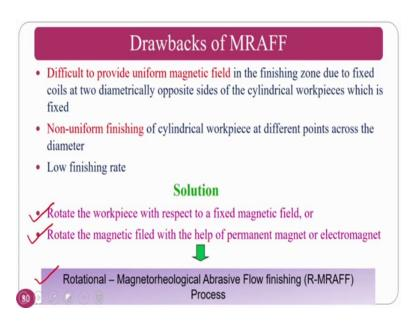
It is difficult to provide uniform magnetic field in finishing row zone due to fixed coils and two dimensional opposite side that means, that if at all I want to finish a cylindrical hole. If I have two electromagnets the magnetic field will be very good on this side and this side, but not on this sides for that purpose you have to rotate the magnetic field; whenever you rotate the magnetic field you can easily finish the cylindrical surfaces.
