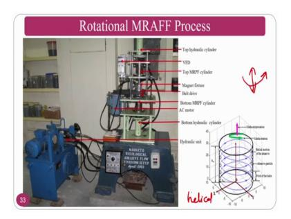
And this is the same set up that is developed by Sunil Jha which is amended the rotary motion by Professor Manas Das who is working currently at IIT Guwahati. So, the rotary motion is provided here to the magnetic field and the cylindrical surfaces are finished.
