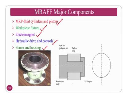
And the major components of this one is MR fluid cylinders and piston, work piece fixture, electromagnet, hydraulic drives and controls and frame and housing these are the sum of the components wherein, you are going to see in this particular slide is MR fluid cylinder. Where you can put the this particular fluid and you can also holds the piston also so that it will retain inside the medium cylinder.
