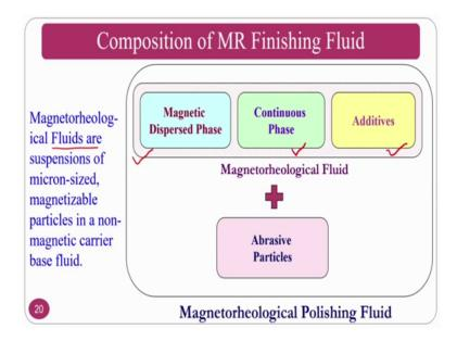
The composition of MR fluid if you see the magnetorheological fluids are exactly same that you are going to see, that you have seen in the MR fluid. As I previously mentioned that you are using the AFF setup along with a MR fluid.
