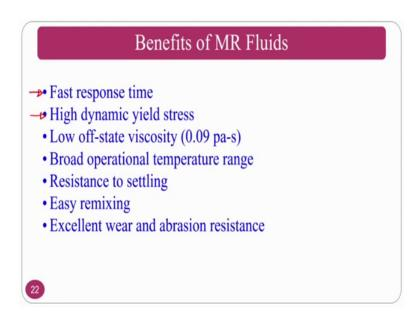
Benefits of magnetorheological fluids, the fast response time these are very responsive within no time this will respond, high dynamic yield stress is another advantage low off state viscosity, broad operational temperature range, resistant to settling, easy remixing, excellent wear and abrasion resistance. These are the few benefits of magneto rheological fluids.
