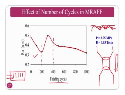
So, we will see, now we will see in the effect of number of cycles as I mentioned cycle means like if you are going to have two strokes that means, at one cycle. So, this is your work piece wherein you have fixture so one time coming is one stroke and going back is another stroke.
