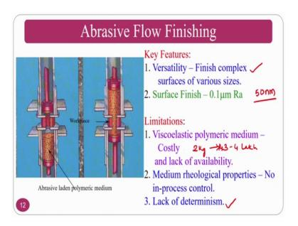
The key features of this abrasive flow finishing versatility it can finish the complex surfaces and it can finish up to 0.1 normally the best surface finish can be achieved is 50 nanometers using this one. So, these two limitations can be improved, so limitations viscoelastic polymer medium is costly normally the cost it will be like in Indian scenario. So, 2 kgs is approximately like 3 to 4 lakhs or sometimes it will be 5 lakhs also.
