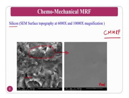
So, at the same time you can see here silicon initial surface and final surface, this is the initial surface and this is the final surface and how the surface is transformed from one surface to another surface. In case of silicon especially the thing is that you can go by water based fluids because water will interact with the silicon and water will act as a chemical.
