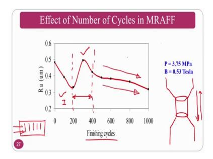
That that is why as the number of cycles increases the finishing will improve that means, that R a value will decrease. And only the new thing about this particular graph which is personally which I like is that the novelty is lying in between 200 to 400 where even though you are increasing the number of cycles the surface roughness is increasing which is against the nature, but there you have to study about the surface morphology, scanning electron microscopy images and other things.
