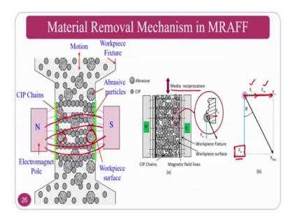
As I was saying material removal mechanism whenever you have a North to South Pole chains formation is there what is going to happen is you are abrasive particles are held, and this abrasive particles along with CIP particles chains will be reciprocated by the hydraulic power.
