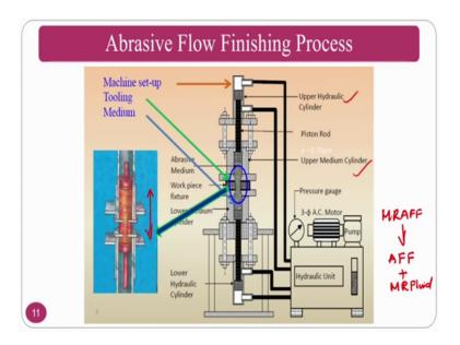
The at the same time if you see the abrasive flow finishing process as we have seen since, why we are seeing the abrasive flow finishing process is this is the MRAFF process is a blend of MRF process and abrasive flow finishing process that is why we are seeing this particular process also. So, the MRAFF process follows the similar structure of AFF process, but only thing that you are going to change is the fluid.
