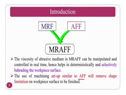
So, introduction to this particular process as I said this is a blend of MRF process that means, that this is one of the hybrid, second hybrid version of MRF process. Where it is blending with abrasive flow finishing process and it is turning out to be
