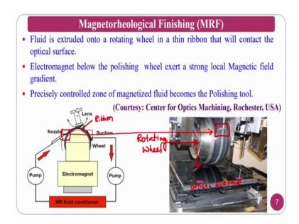
Magnetorheological finishing process; as you can see here, the schematic diagram and experimental setup both are there. So, fluid is extruded into the rotating wheel in a thin ribbon that will contact the optical surface; that means, that this is my optical surface, this is my optical surface and this is my rotating wheel ok.
