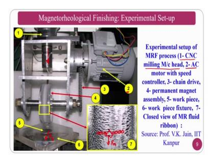
So, if you see the juned version of this particular process, where the work piece is there the 5 stands for work piece. So, the one is nothing but the CNC milling head, basically the experimental setup is developed on the end milling process ok. So, it is not too
