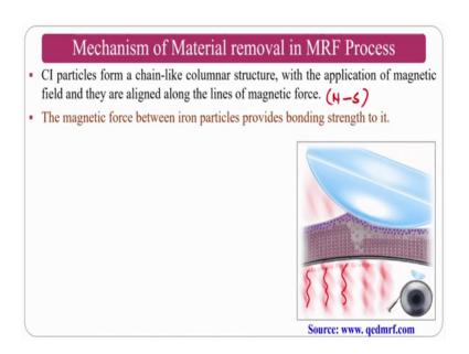
I mean to say the solid ribbon. So, mechanism of material removal in MR finishing process is carbonyl iron particles from the chain like columnar structures that you have seen in the previous slides; with application of the magnetic field they align along the lines of magnetic force from north pole to south pole. The magnetic force between iron particles provide the bonding strength to the MR-fluid. And you can see here the animation where the magnetic field is applied like this, ok.
