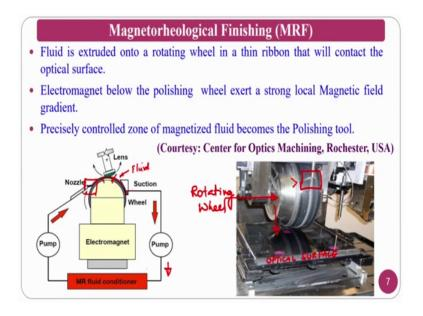
So, the yellow portion, here is the magnet that one can keep ok. Once it crosses that this particular location, again it will become a fluid. And this fluid will suck by sucking pump and it will supply to the magnetic fluid conditioner so that it can recycle ok. In the magnetic fluid conditioner, you can have some other magnet so that the chips all will be attracted towards that one, and whenever you are pumping again the chips will not be
