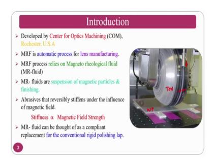
So, introduction to MRF process see this is how the MRF process works. This is the workpiece and this is the tool where the fluid is dispensed here. And because of the magnetic field that is there inside the grinding wheel, it becomes a thin ribbons type of structure and this is called a flexible polishing belt or you can say flexible polishing ribbon.
