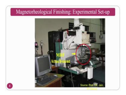
So, this is what the magnetorheological finishing setup that is developed by a Professor VK Jain at IIT, Kanpur.
