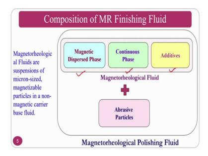
The composition, this is the most important thing for the MR-fluid, because you should know: what are the ingredients that are there. How the abrasive particles are getting assistance. As you have seen in the abrasive flow finishing process that the polymer chains along with the plasticizer softeners, this will support by giving the visco elastic nature to the abrasive particle, but how you are going to get that type of support in this one.
