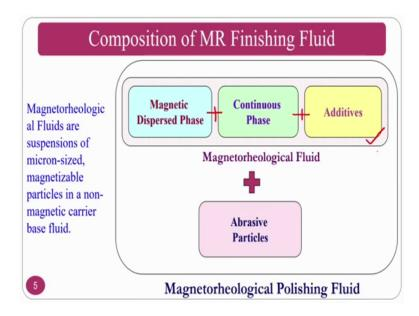
So, magnetic phase particles, plus continuous phase plus additives gives you a suspension; which is a liquid because you have to jet this liquid so that it will form the chains ok. So, in a liquid there will be a density difference. Once you add the abrasive particles ok, what you are going to add for this one is abrasive particles.
