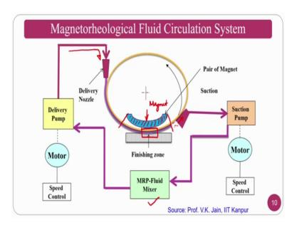
You can see here the magnetorheological fluid circulation system. You have a speed control motor will be there delivery pump; that means, that it will deliver the fluid from the conditioner tank like this, and it will enter into the finishing region. As you can see here this is a sky blue one is a magnet. From this region to this region, the fluid will act as a thin ribbon. Beyond which what is it is going to happen is that it will not act as a ribbon ok.
